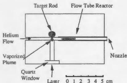
Figure 1. Schematic diagram of vaporization source and flow tube reactor
