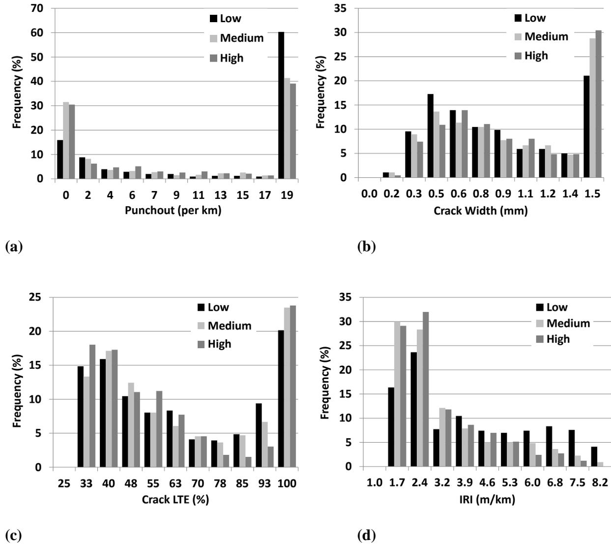
Fig. 5. Distribution of CRCP predicted distresses under cold-dry (CD) climate zone: (a) punchout, (b) crack width, (c) crack LTE, and (d) IRI.
