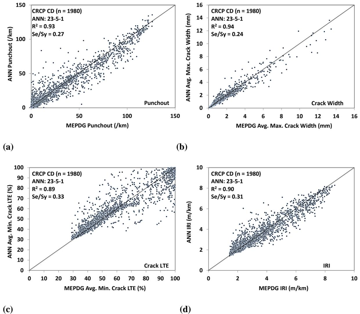
**Fig. 6. ANN predicted vs. MEDPG predicted CRCP distresses under cold-dry (CD) climate zone: (a) punchout, (b) crack width, (c) crack LTE, and (d) IRI.**
