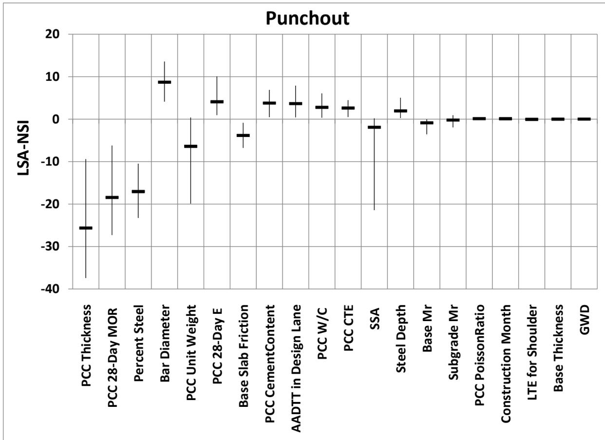
Fig. 2. LSA-NSI values for punchout in CRCP.
