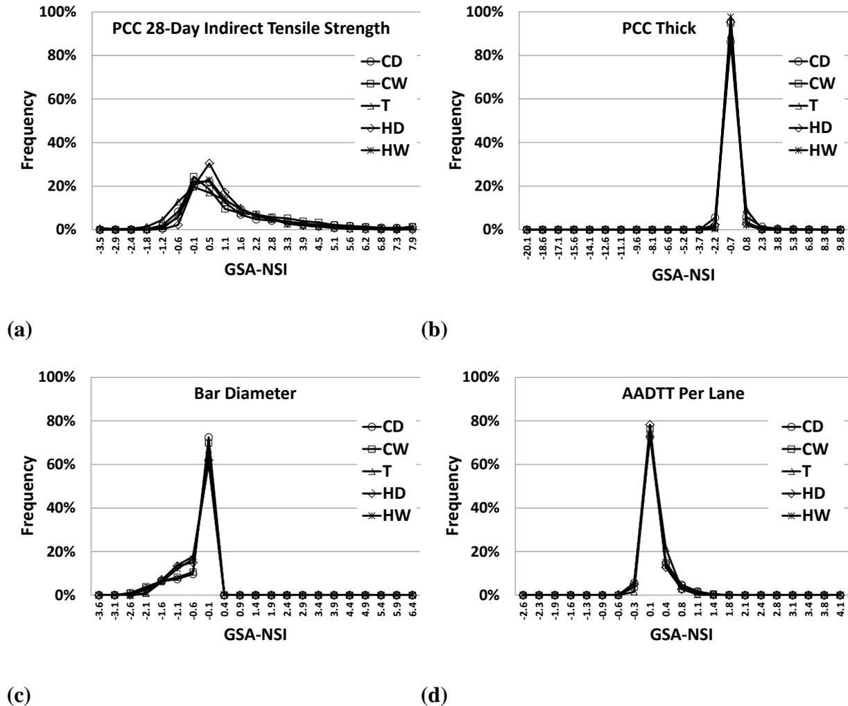
**Fig. 7. Distributions of GSA-NSI values for JPCP: (a) punchout by PCC 28-Day indirect tensile strength, (b) crack width by PCC thickness, (c) crack LTE by bar diameter, and (d) IRI by AADTT per lane.**
