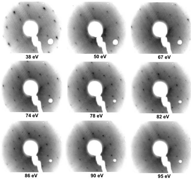
FIG. 2. LEED patterns of 1.2 ML Na grown on *i*-Al-Pd-Mn surface at several incident electron-beam energies. Images are shown in inverted gray scale where black indicates the highest brightness. All the LEED patterns have been recorded at 130 K.
