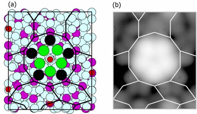
FIG. 5. (Color online) (a) Pentagonal  $\text{Pb}_5$  clusters on the five-fold surface of *i*-AlPdMn. The black circles represent the positions of Pb adatoms in the  $\text{D5T}_0$  cluster. The large green (pale) circles show the positions of Pb adatoms in the  $\text{D5R}$  cluster. Other circles represent atoms of the surface, cf. Fig. 4. (b) The calculated STM image of the  $\text{D5R}$  cluster.
