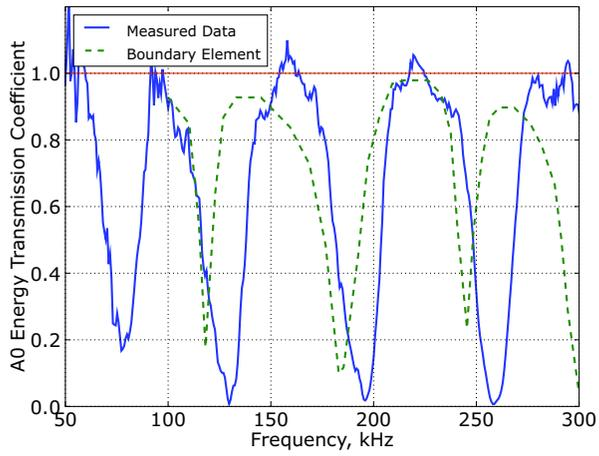
**FIGURE 5.** Comparison of measured and calculated energy transmission coefficients for high aspect-ratio 0.8 inch tall  $\times$  0.1 inch wide stiffener.
