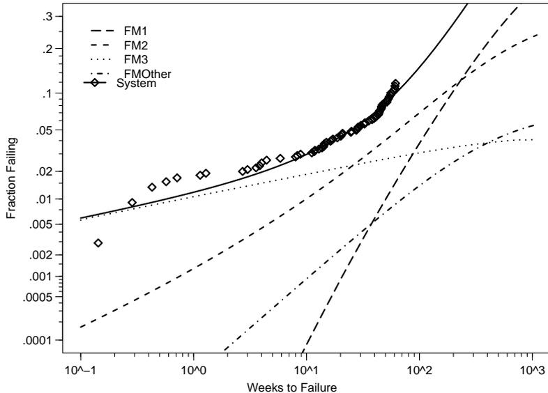
Figure 5: Lognormal probability plot of the system failure times along with the ML estimate of the series system failure-time cdf for the not-connected population. The ML estimates of the sub-distribution functions for the not-connected population are also shown.
