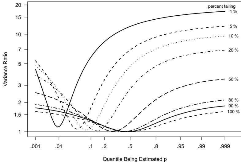
Figure 13: Comparisons of the asymptotic variance ratio for estimating lognormal  $t_p$  for different percentage failing.
