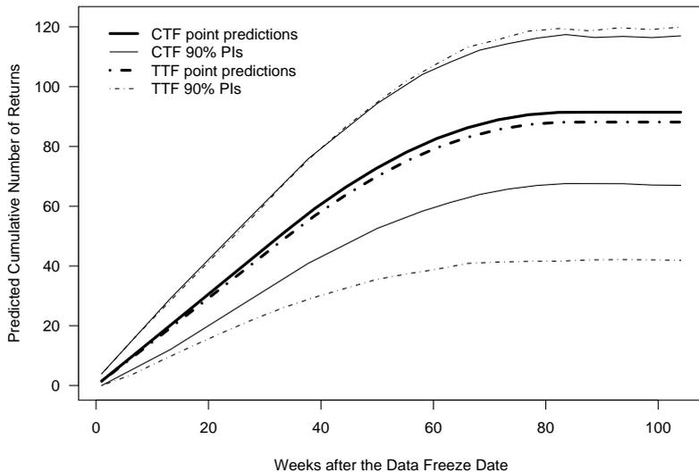
Figure 12: Comparison of prediction result for the failure-time data results and cycles-to-failure data for the not-connected population.
