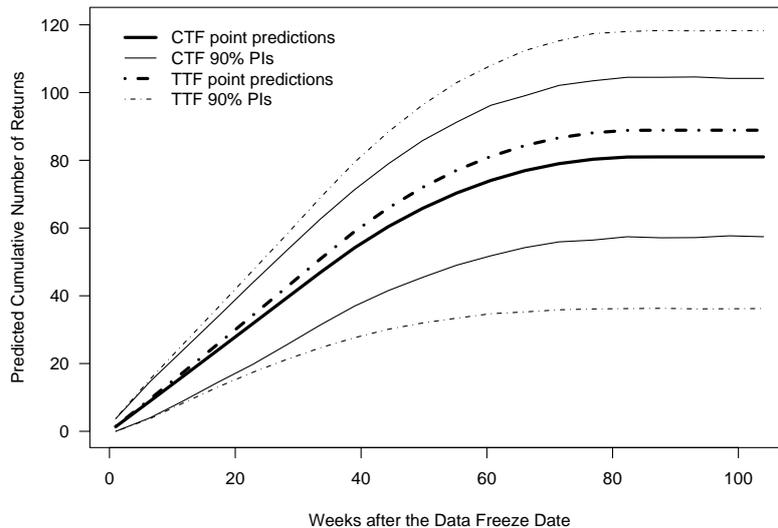
Figure 11: Comparison of prediction result for the failure-time data results and cycles-to-failure data for the connected population.
