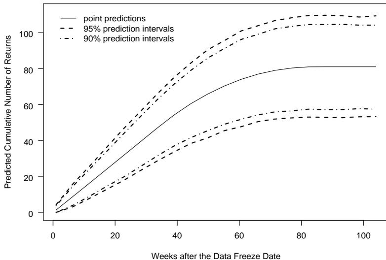
Figure 8: The point predictions and pointwise PIs for the cumulative number of returns as a function of time after the DFD for the connected population.
