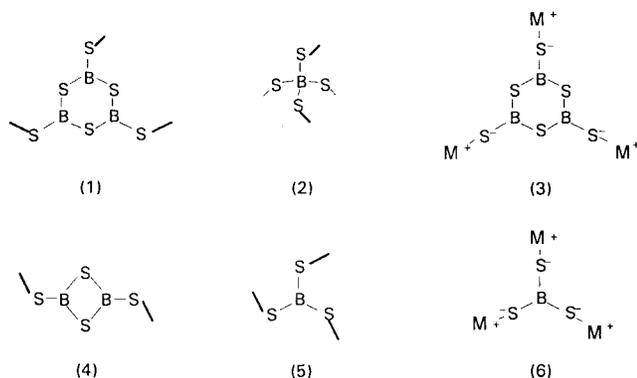
**Figure 1.** Proposed structural units found in alkali thioborate compounds: (1) thioboroxyl six-membered ring; (2) tetrahedral ( $\text{BS}_4$ ) unit; (3) metathioborate; (4) four-membered ring; (5) trigonal ( $\text{BS}_3$ ) unit; and (6) orthothioborate.
