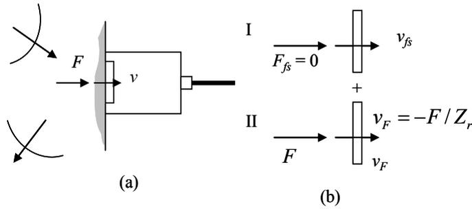
**FIGURE 2.** (a) A contact receiving transducer, and (b) the decomposition of the reception process into problems I and II. In problem I the surface is completely free and the incident waves are present while in problem II the incident waves are absent and the force,  $F$ , acting on the transducer face is present.
