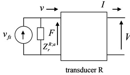
**FIGURE 3.** A lumped parameter model of a contact receiving transducer as a “mechanical current” source in parallel with the acoustic radiation impedance of the transducer.
