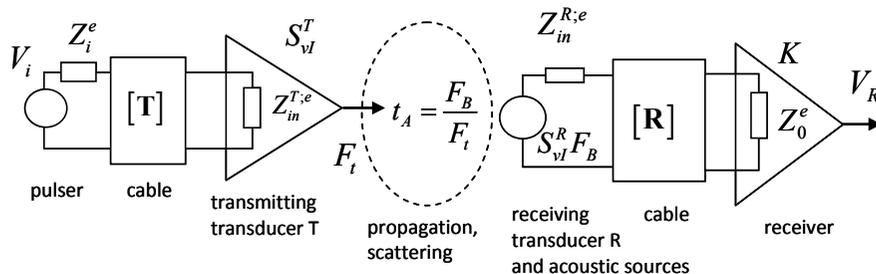
**FIGURE 1.** Elements of an electroacoustic measurement model for an ultrasonic immersion setup.
