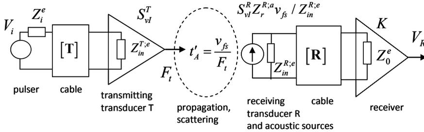
**FIGURE 4.** Elements of an electroacoustic measurement model for an ultrasonic contact testing setup.
