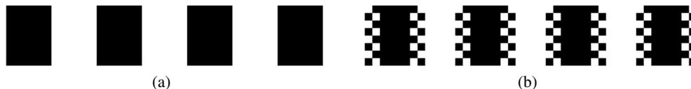
Figure 2. Example of conventional squared binary pattern and the modified pattern. (a) traditional squared binary pattern; (b) 2D area-modulated binary pattern.
