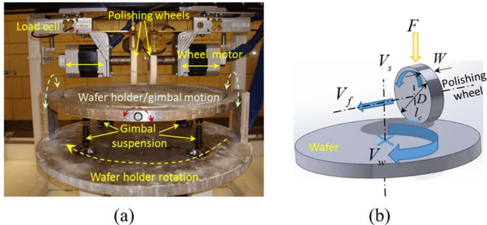
Figure 1: (a) Optical view of the PPP system showing the relative motion of the main components (dashed arrows). Vertical crosshead provides down feed. Polishing wheels translational stages provides transverse feed and table rotation provides progressive whole surface polishing. (b) Illustration of the obliqueness in process kinematics
