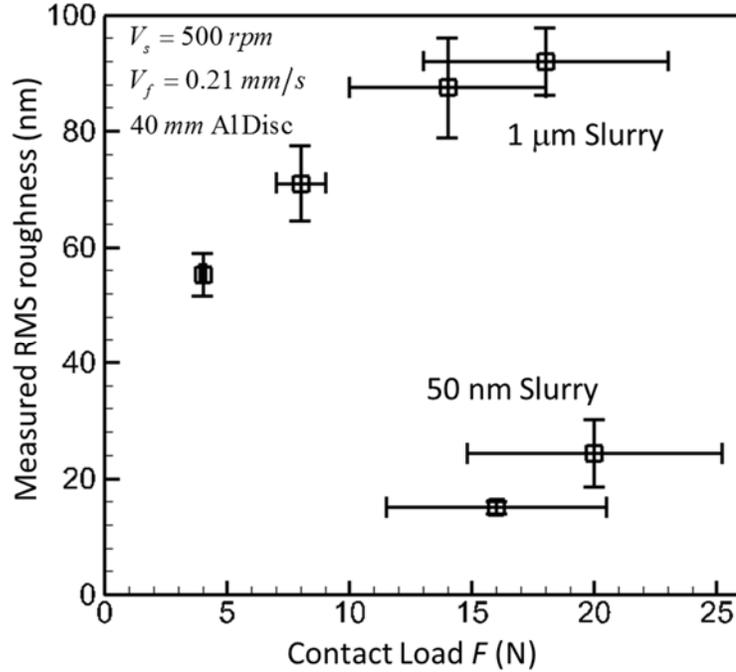
Figure 7: Role of applied contact load on the variation of RMS roughness, showing persistent increase with the load. RMS roughness is measured over an area of  $1.4 \times 1.4 \text{ mm}^2$
