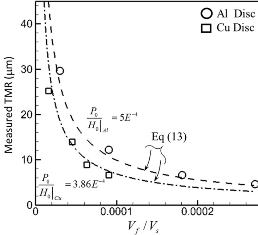
Figure 10: Process domain summarizing the entire data set for different process and material parameters. A parametric correlation can be identified for each material system, similar to the phenomenological Preston-type polishing relationship.
