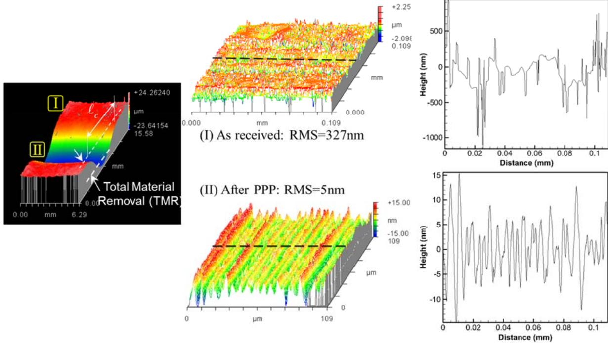
Figure 5: Polishing results of 40 mm Cu-disc using 1  $\mu\text{m}$  slurry, showing local from RMS=327 nm to less than RMS=5 nm after a single PPP sweep.
