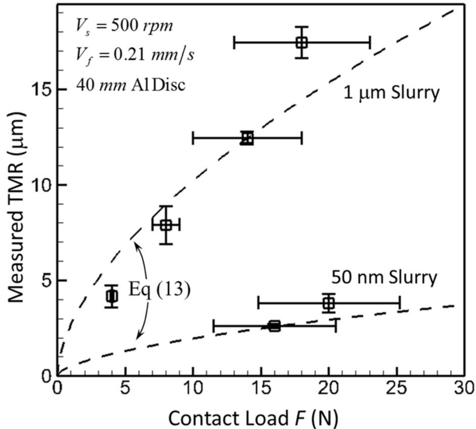
Figure 6: Role of applied contact load on the variation of TMR. The model prediction of Eq. (13) remarkably fit the experimental data with scaler of order unity for slurries with two different abrasive sizes.
