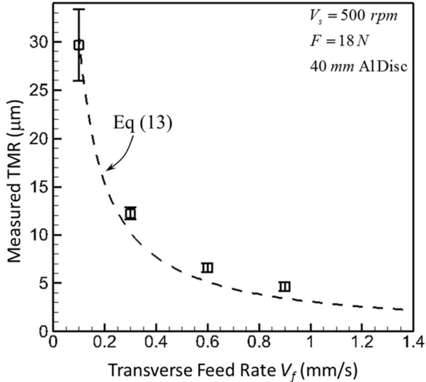
Figure 8: Role of transverse feed rate on the variation of TMR, showing a marked reduction due to the dwell time reduction. The model prediction of Eq. (13) remarkably show the inverse proportionality with  $V_f$ .
