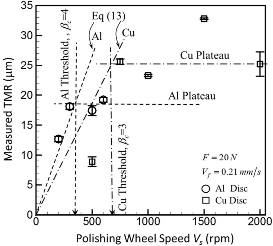
Figure 9: Role of polishing wheel speed on the variation of TMR, showing an initial increase in TMR up to 1000 rpm, TMR independent trend. The hypothesized domain of validity of the model Eq. (13) is also shown.  $\beta_c \approx 2 - 4$  is a scaling factor that defines the distance between two overlapping ploughed trenches.
