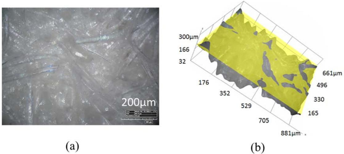
Figure 2: Topology of the utilized polishing wheel. (a) Optical micrograph of the surface topology. (b) Three dimensional optical micrograph of pad asperity, showing the pad density,  $\xi_{asp}$  at a critical height of three times the asperity radius (shaded plane).
