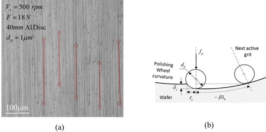
Figure 3: (a) Polished Al surface with 1  $\mu\text{m}$  slurry showing effective cutting length along  $v_s$  direction is about 250  $\mu\text{m}$ . (b) Sketch of the proposed active cutting grit, and the shadow trail of length  $\beta\lambda_p$  in its wake, until a new grit penetrate the surface, ( $\beta \sim 50$  for  $d_p = 1 \mu\text{m}$ ).
