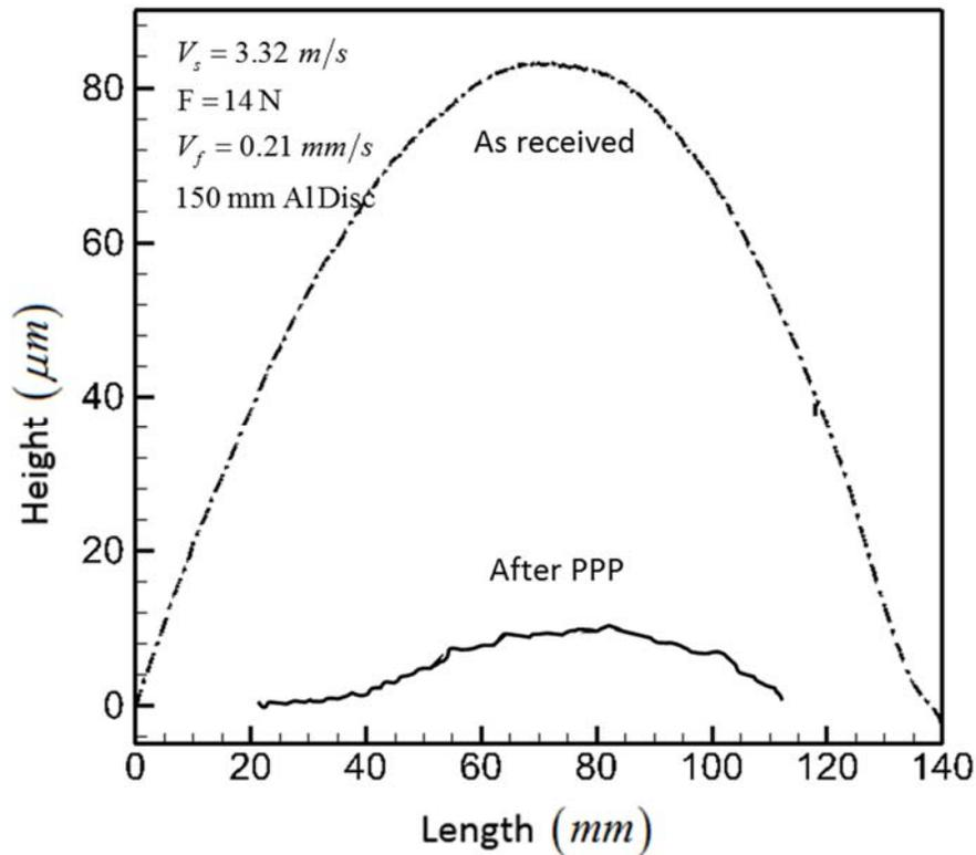
Figure 4: Evolution of total thickness variation (TTV) over 150 mm Al-disc after a single sweep of the surface on the PPP platform showing reduction of TTV from more than 80  $\mu\text{m}$  to less than 12  $\mu\text{m}$ . Table rotated at 50 rpm.
