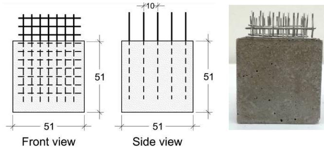
Figure 1. Geometry (left and middle) and sample picture (right) of cement-based nanocomposite specimens
