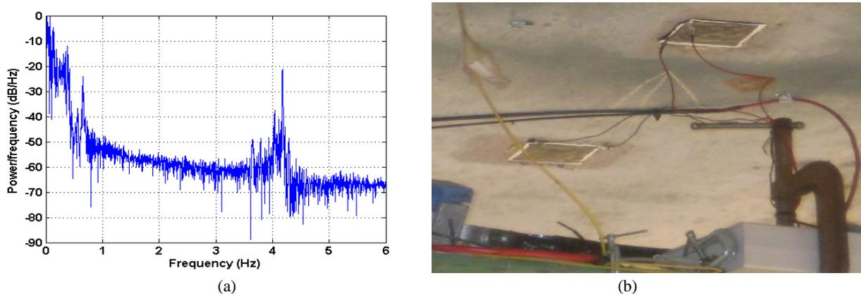
Fig. 4. (a) Power Spectra Density of the Capacitance Signal; and (b) Two Sensing Patches Deployed Under the Deck [12].
