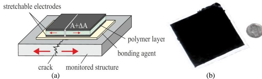
**Fig. 1.** (a) Schematic of Sensing Principle [14]; and (b) a Sensing Patch, 75 x75 mm (3 x 3 in).
