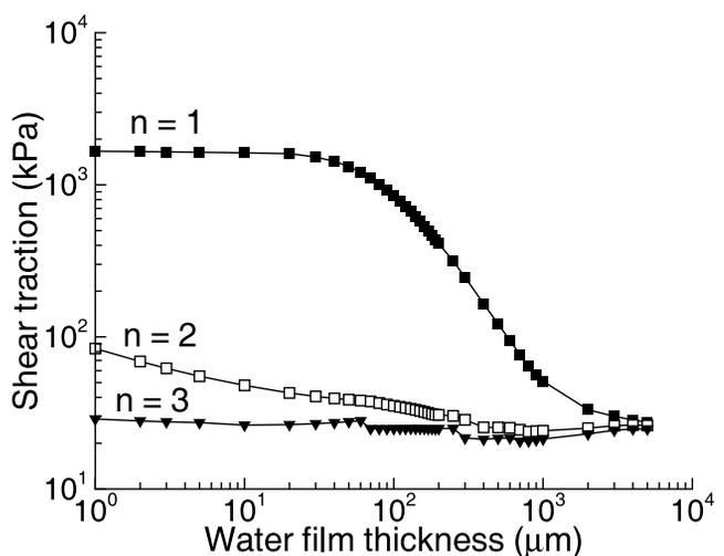
**Figure 8.** Shear traction as a function of water film thickness for  $n = 1, n = 2,$  and  $n = 3$  for conditions at Engabreen.
