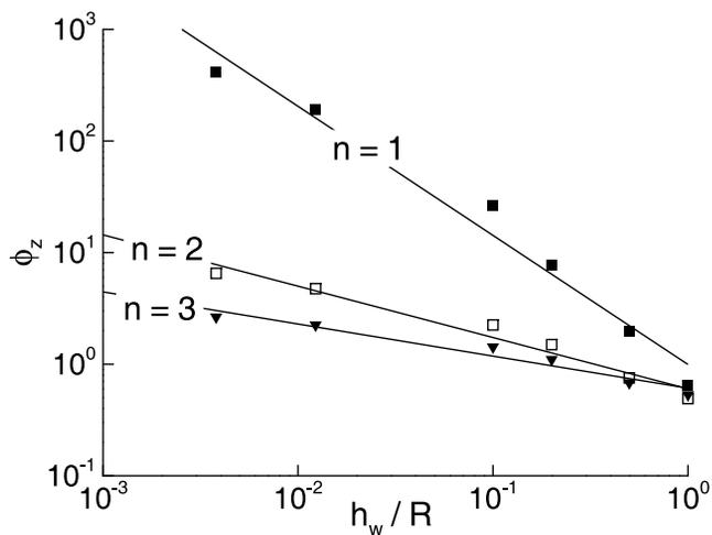
**Figure 7.** Variable  $\phi_z$  as a function of dimensionless ratio  $h_w/R$  for  $n = 1, 2,$  and  $3$ . Each symbol represents a numerical solution. Lines are power law fits.
