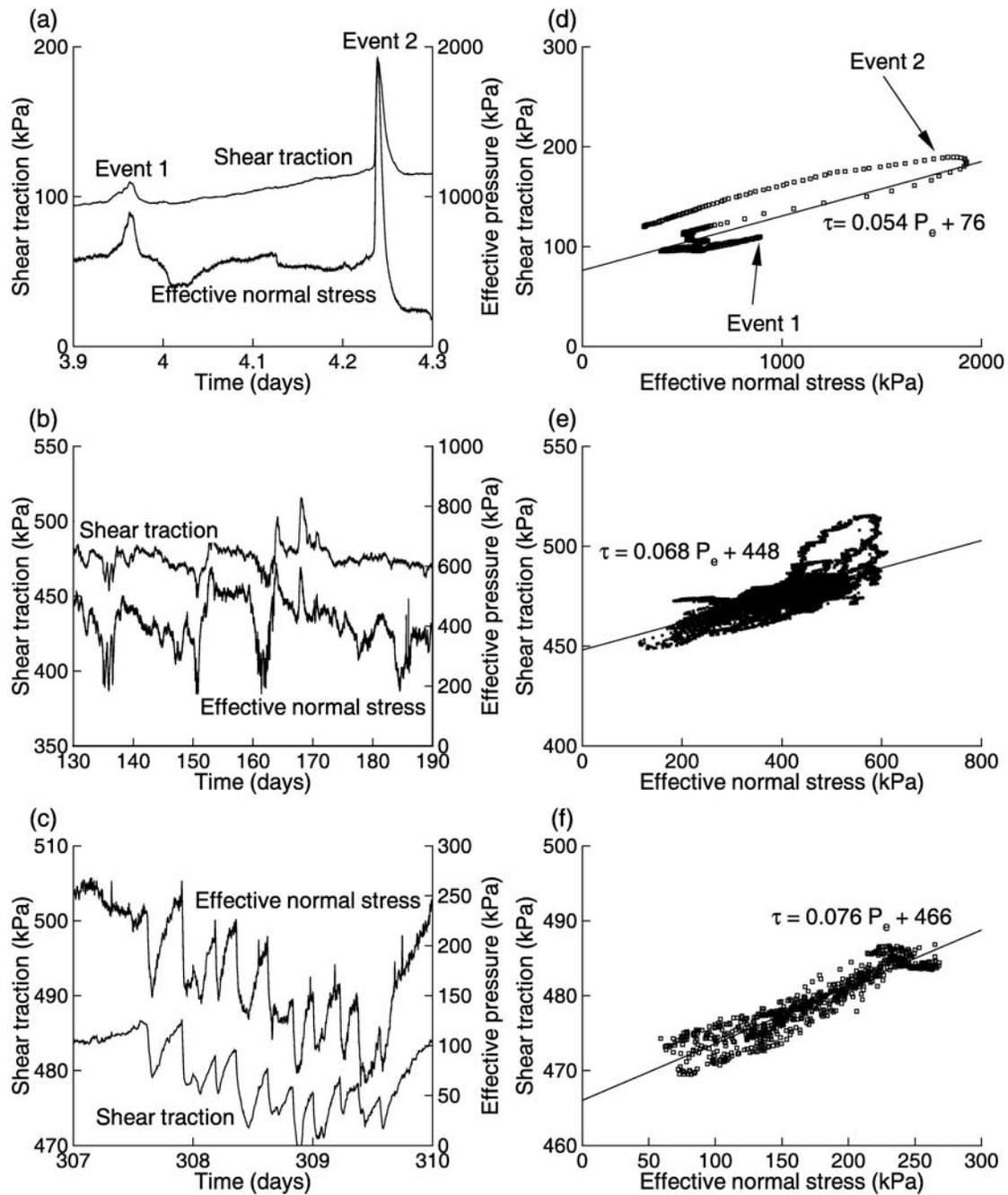
**Figure 4.** Selected time series of shear traction and effective normal stress in (a) 2002, (b, c) 2003, and (d, e, f) associated plots of shear traction versus effective normal stress. Data are unsmoothed.
