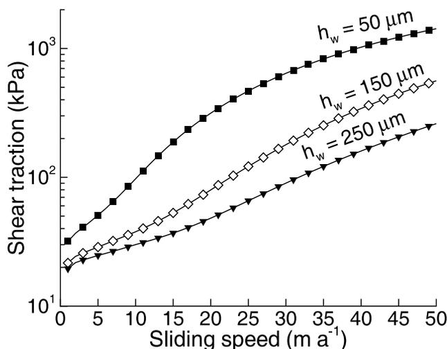
**Figure 13.** Shear traction as a function of sliding speed for  $v_{\text{geo}} = 0.006 \text{ m a}^{-1}$  and  $p_e = 300 \text{ kPa}$ . The particle size distribution is given in Table 2.
