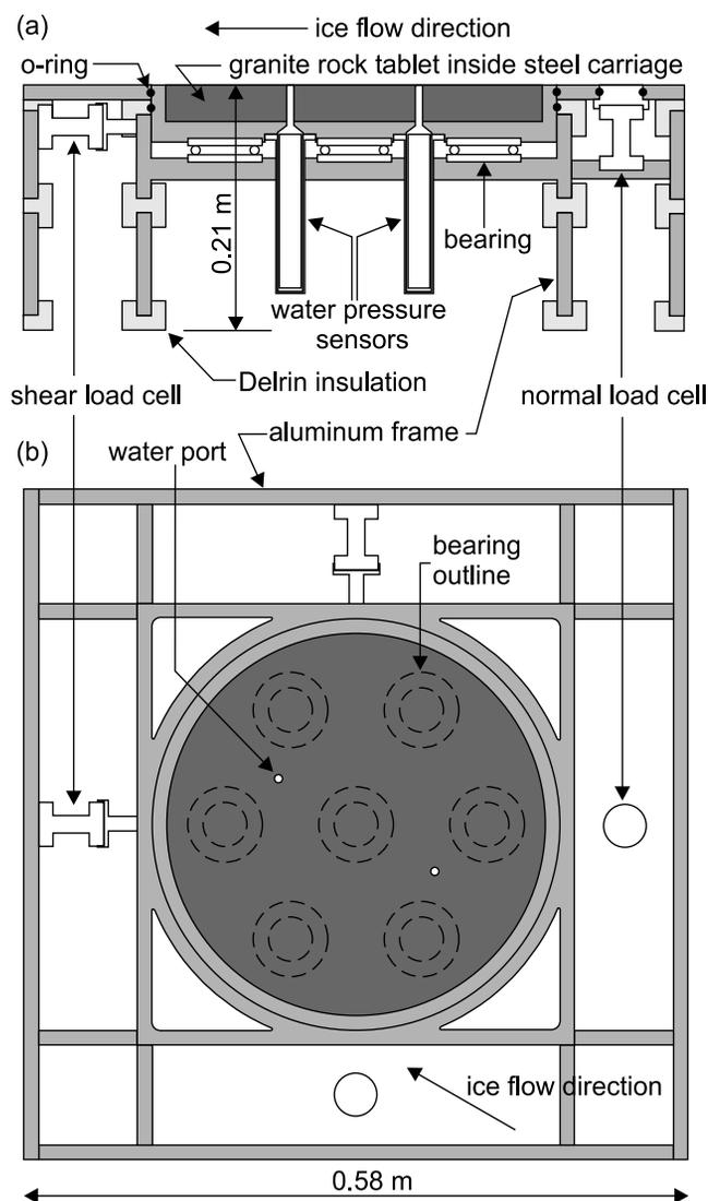
**Figure 1.** Schematic of panel: (a) side view and (b) top view.
