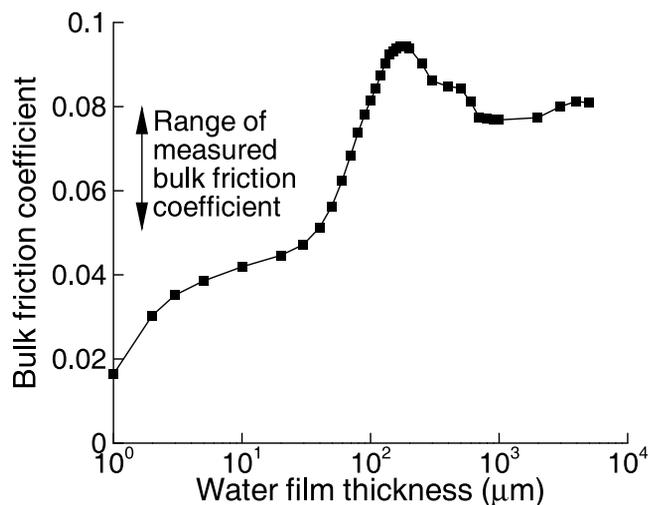
**Figure 10.** Computed effective friction coefficient between dirty basal ice and bedrock as a function of water film thickness.
