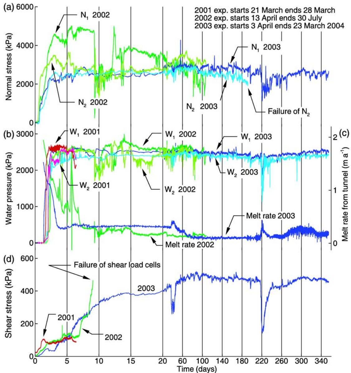
**Figure 2.** (a) Normal stresses  $N_1$  and  $N_2$  between the ice and the panel, (b) water pressures  $W_1$  and  $W_2$  at the panel surface, (c) melt rate due to heat flux from tunnel, and (d) shear stress measured in 2001 (red curves), 2002 (green curves), and 2003 (blue curves). The time axis is split into two different scales. Data are unsmoothed.
