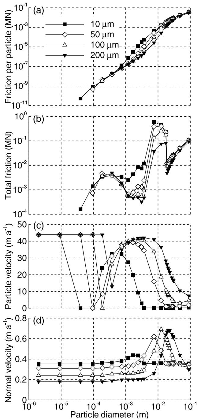
**Figure 9.** (a) Frictional force per particle of a given class size (given diameter), (b) total frictional force of particles in a given class size, (c) particle velocity, and (d) bed-normal ice velocity as a function of particle diameter for four different water film thicknesses (10, 50, 100, and 200  $\mu\text{m}$ ) and  $p_e = 300$  kPa.
