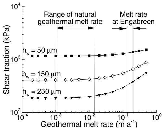
**Figure 12.** Shear traction as a function of geothermal melt rate for  $U = 43.8 \text{ m a}^{-1}$  and  $p_e = 300 \text{ kPa}$ . The particle size distribution is given in Table 2.
