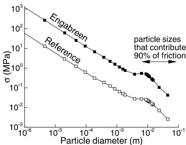
**Figure 11.** Computed stress in ice flowing around particles,  $\sigma$ , as a function of particle radius for two cases: Engabreen and a glacier with  $U = 10 \text{ m a}^{-1}$ ,  $h_w = 50 \mu\text{m}$ , and  $p_e = 300 \text{ kPa}$ . The particle size distribution is identical in the two cases.
