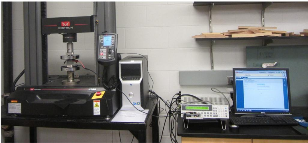
Figure 3: Setup for strain sensing tests.
