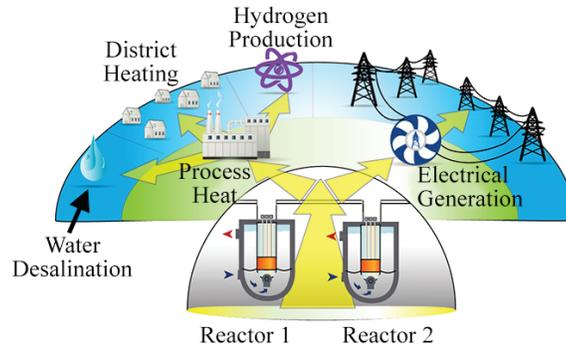
**FIGURE 1.** AdvSMR Deployment Concept Illustrating Multiple Generation Missions.
