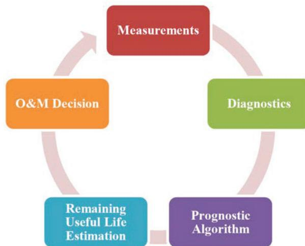
**FIGURE 3.** Depiction of the Multiple Components of a PHM System for Passive AdvSMR Components.
