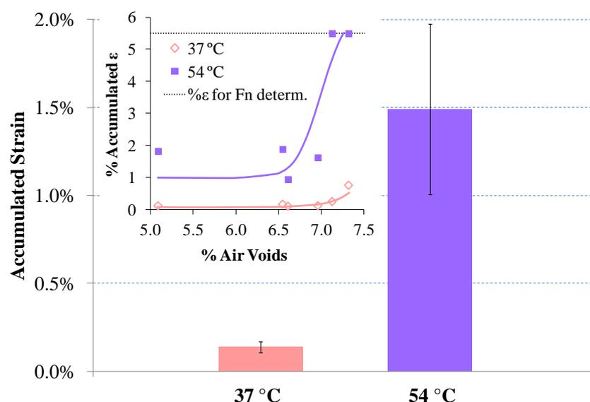
Figure 10. Accumulated strain at 10,000 cycles for the 7% air voids mixture
