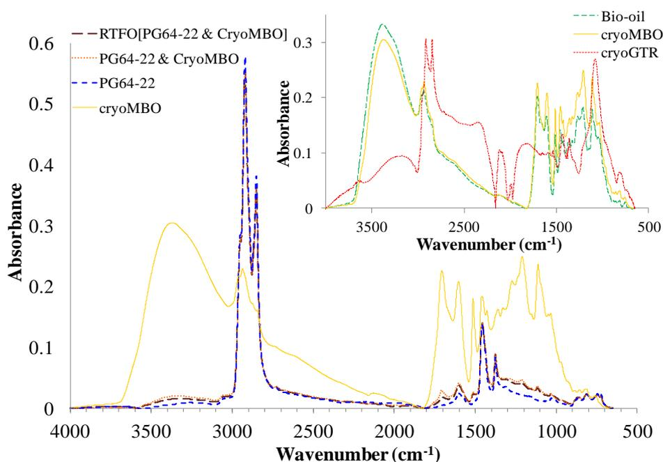
Figure 5. FTIR spectra of different binder constituents
