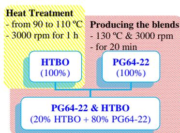
Figure 2. Production of the PG64-22 & HTBO
