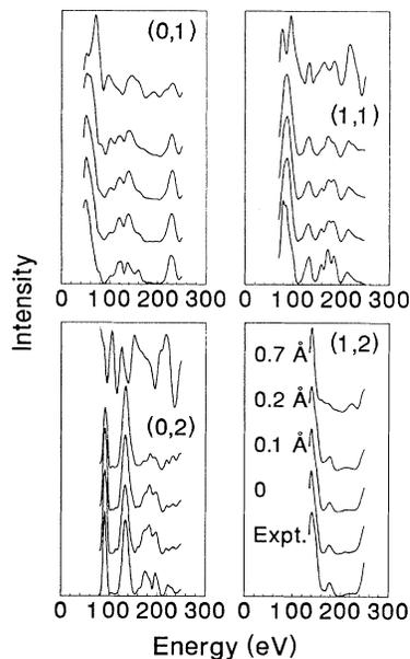
FIG. 3. Representative comparison between experimental  $I(E)$  curves and best-fit theoretical  $I(E)$  curves for  $\sigma=0, 0.1, 0.2,$  and  $0.7 \text{ \AA}$ . Note the wide range of response with respect to  $\sigma$ .
