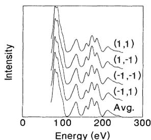
FIG. 1. Comparison between experimental  $I(E)$  curves for the (1,1) beam set and their average at normal incidence. Curves are collected at 105 K.
