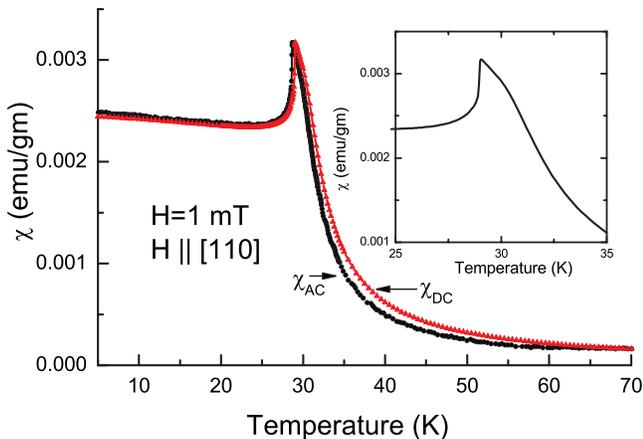
FIG. 2. (Color online) Magnetic susceptibility  $\chi = M/H$  of MnSi as a function of temperature. Measurements were made in a field of 1 mT. The ac susceptibility data were scaled by simple multiplication.
