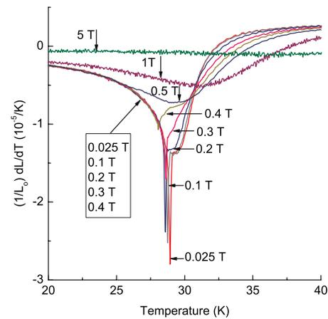
FIG. 5. (Color online) Linear thermal expansion coefficient of MnSi near the phase transition in magnetic fields ( $\mathbf{H} \parallel [110]$ ). It is seen that moderate magnetic fields up to 0.4 T do not influence thermal expansion of the helical phase.
