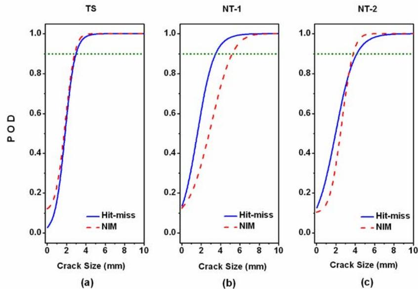
FIGURE 5. POD comparisons between hit/miss and NIM methods for rivet holes at TS (a), NT-1 (b) and NT-2 (c).
