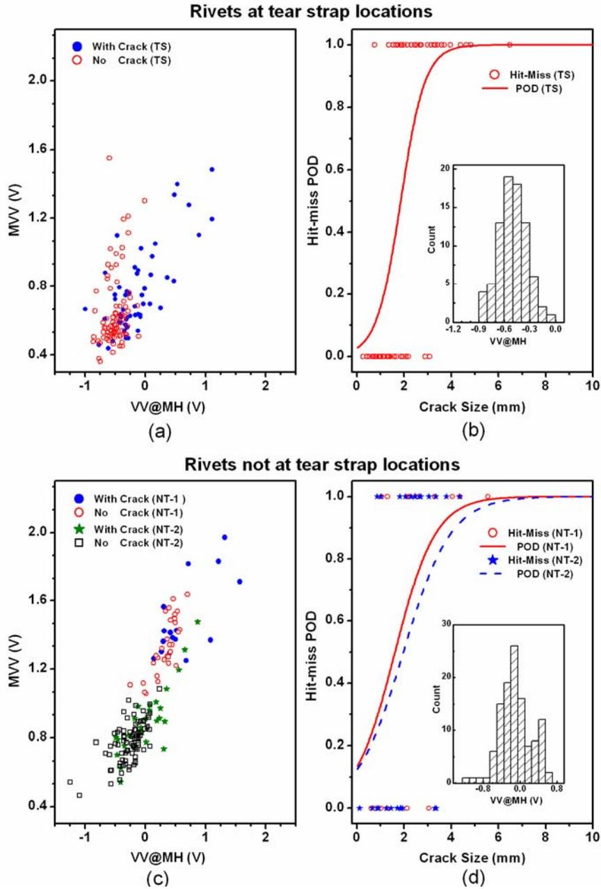
FIGURE 2. The relationships between MVV and VV@MH are shown for TS (a) and NT (c) with solid symbols representing rivet holes with a crack and open symbols representing rivet holes without a crack. The Hit/Miss PODs are shown in (b) for TS and in (d) for NT, where the Hit/Miss decisions are indicated as zero (miss) and one (hit). The noise distribution of VV@MH for both locations are plotted in the inset of (b) for TS and of (d) for NT.
