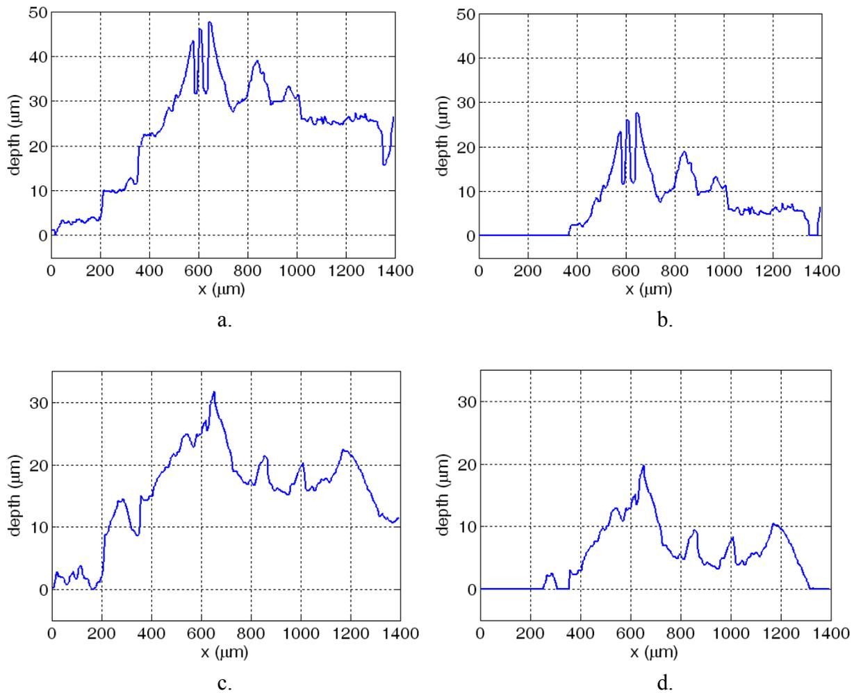
Figure 5: Comparison of generated height differences of virtual marks from a) 30 degree angle, high applied force; b) 30 degree angle, low applied force; c) 45 degree angle, high applied force; d) 45 degree angle, low applied force.
