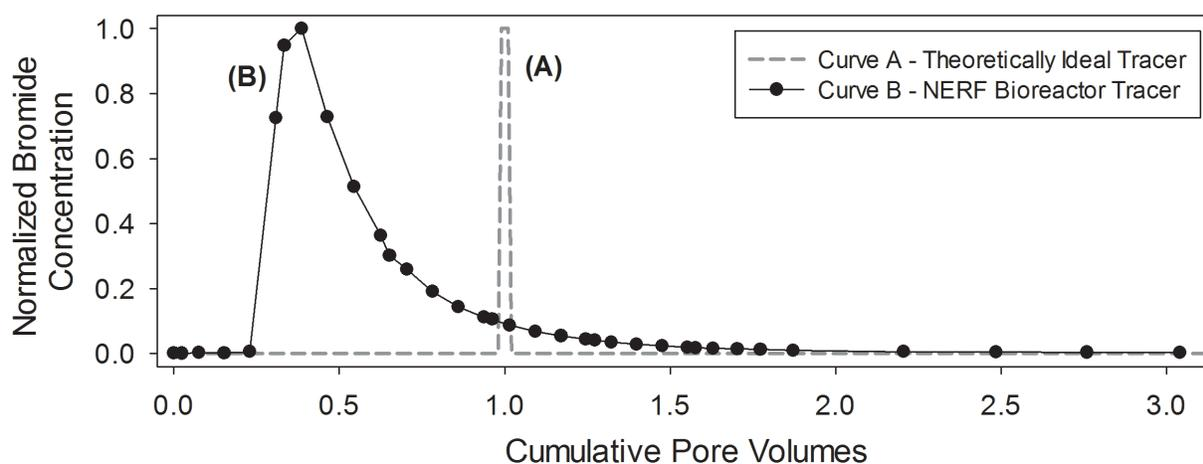
**Figure 1. Tracer testing curve for a theoretically ideally performing reactor (A) and for the ISU Northeast Research Farm bioreactor test in May 2011 (B). Bromide concentration normalized to peak concentration in each case.**
