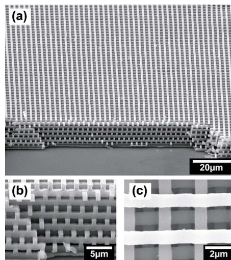
FIG. 3. (Color online) SEM micrographs of a 12-layer titania PC. Tilted SEM image of a cleaved edge at (a) lower and (b) higher magnifications; (c) top view.
