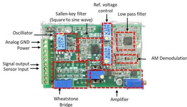
Figure 4. Top view of prototype capacitance sensor board
