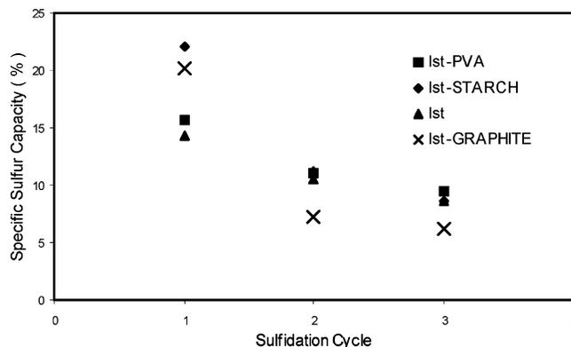
**Figure 11.** Effects of pore-forming additives on reactivity of limestone pellets over multiple cycles of sulfidation and regeneration.
