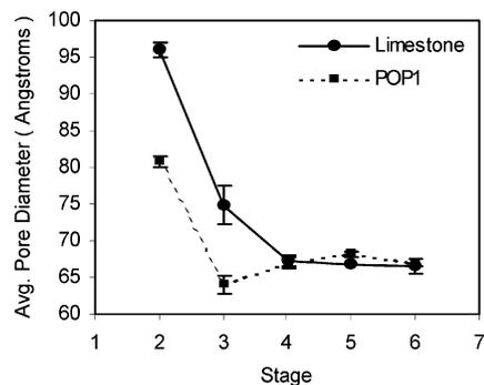
**Figure 4.** Average pore size of limestone and POP1 pellets in the 20–3700 Å range (95% CI).
