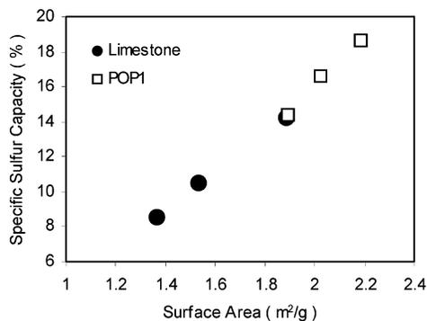
**Figure 10.** Comparison between specific sulfur capacity and surface area for limestone and POP1 pellets. Data taken from three consecutive sulfidation/regeneration cycles.
