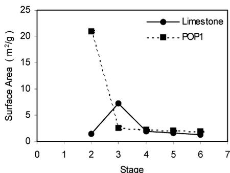
**Figure 3.** Specific surface area of the pellets measured throughout six different stages of processing and reaction (95% CI).
