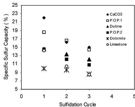
**Figure 12.** Comparison between multiple starting materials in pellet form, over multiple cycles of sulfidation and regeneration.
