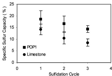
**Figure 2.** Specific sulfur capacity of pellets averaged over multiple cycles of sulfidation and regeneration (95% CI).
