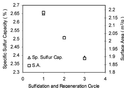
**Figure 9.** Comparison between specific sulfur capacity and surface area of POP1 pellets as a function of consecutive sulfidation/regeneration cycles. Pellets tested in groups of 10.
