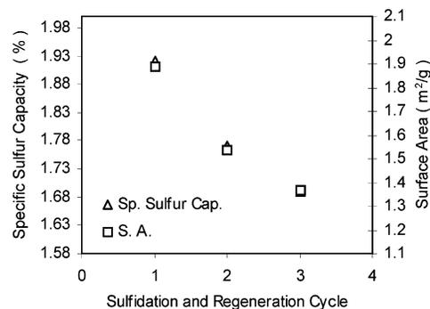
**Figure 8.** Comparison between specific sulfur capacity and surface area of limestone pellets as a function of consecutive sulfidation/regeneration cycles. Pellets tested in groups of 10.
