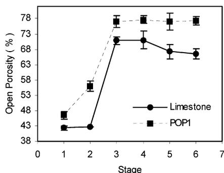
**Figure 7.** Open pore porosity of the pellets throughout the stages of processing and reaction (95% CI).
