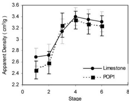
**Figure 6.** Apparent density of the pellets versus number of processing and reaction stage (95% CI).
