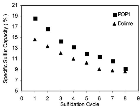
**Figure 13.** Single pellet comparison between POP1 and dolime pellets over consecutive sulfidation/regeneration cycles.
