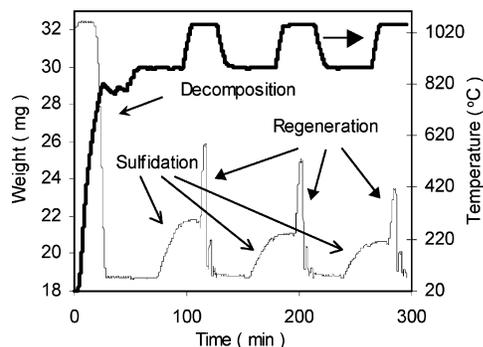
**Figure 1.** Limestone pellet calcined, sulfided, and regenerated through three consecutive cycles.
