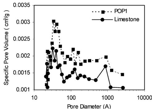
**Figure 5.** Pore size distribution of POP1 and limestone pellets at stage 6.
