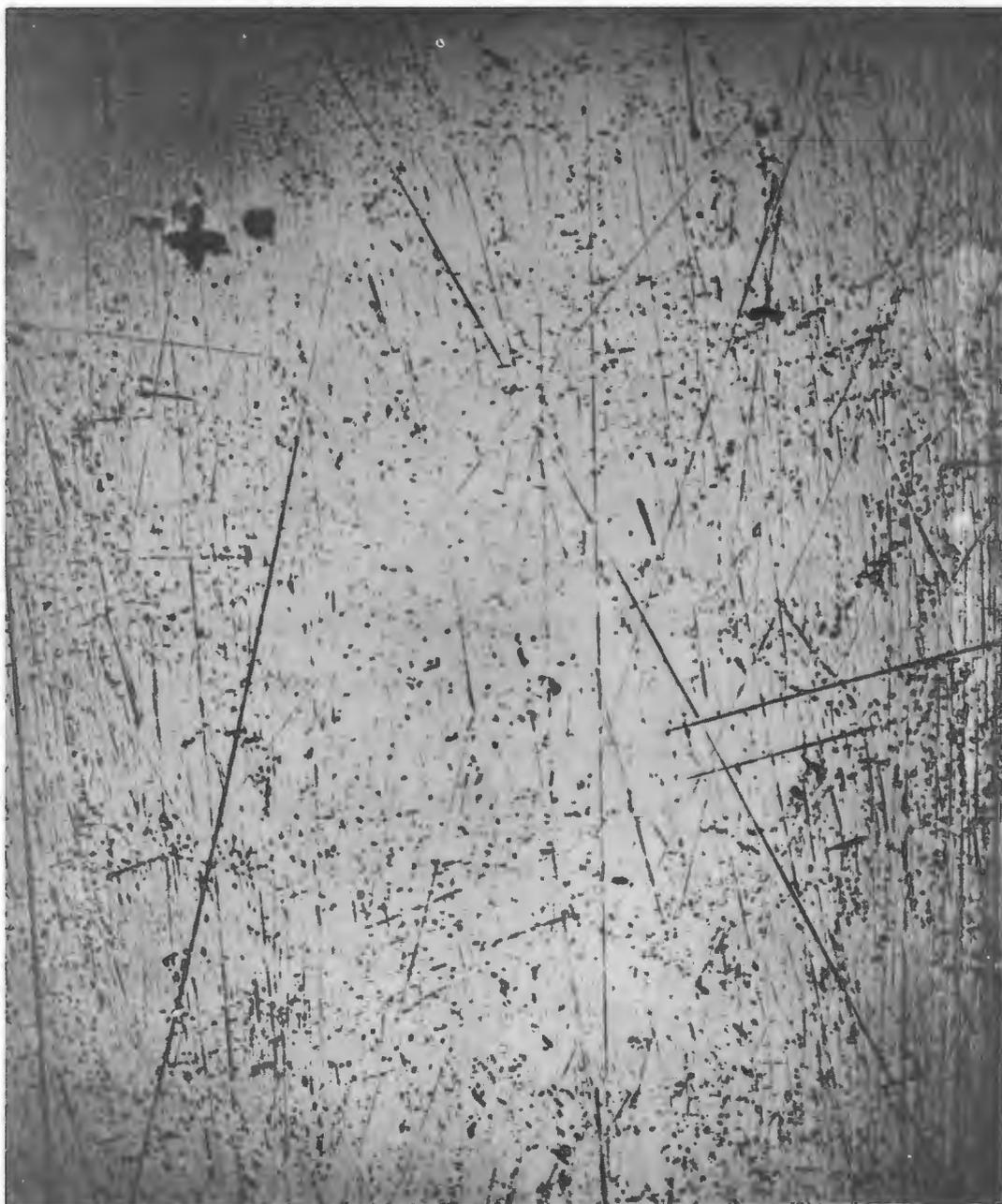
Fig. 13. Microstructure of low carbon region in uranium product due to segregation. Straight lines are scratches in soft metal. 100X.
