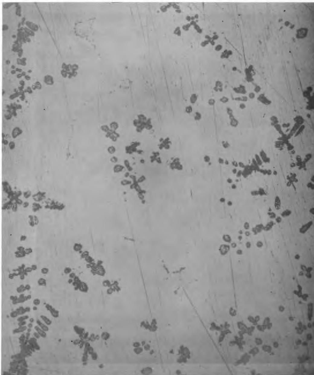
Fig. 11. Microstructure of uranium metal prepared in thoria-yttria crucible. Thorium in metal 200 ppm. 100X.
