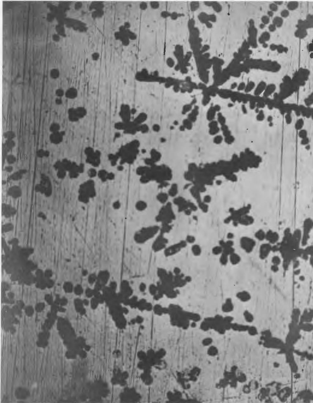
Fig. 12. Microstructure of metal prepared in thoria-yttria crucible. Charge with excess carbon. Thorium in metal 1200 ppm. 100X.
