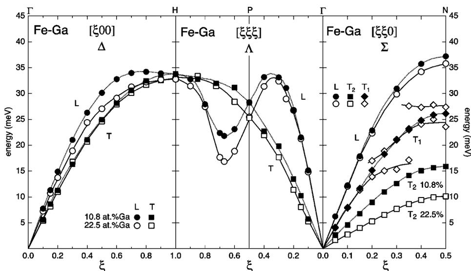
FIG. 1. Comparison of the dispersion curves of Fe-10.8 and 22.5 at. % Ga samples. (The solid symbols are Fe-10.8 at. % Ga and the open symbols are Fe-22.5 at. % Ga.)
