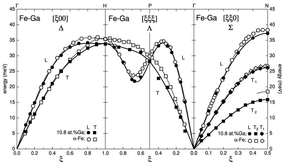
FIG. 2. Comparison of the dispersion curves of Fe-10.8 at. % Ga and  $\alpha$ -Fe (Ref. 6). (The solid symbols are Fe-10.8 at. % Ga and the open symbols are  $\alpha$ -Fe.)
