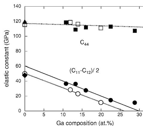
FIG. 4. Fe-Ga elastic constants estimated from the slopes of the phonon dispersion curves for the five Ga concentrations studied and from the Born-von Kármán analysis of Minkiewicz *et al.* (Ref. 6) for  $\alpha$ -Fe (solid symbols). The open symbols are from the ultrasonic measurements of Wuttig *et al.* (Ref. 4).
