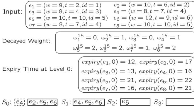
FIG. 1. An example stream with 8 elements arriving in the order  $e_1, e_2, \dots, e_8$ , and its sketch  $\{S_0, S_1, S_2, S_3\}$  for the decayed sum. The current time is 15. The decayed weight of  $e_i$  at time  $t$  is denoted by  $\omega_i^t$ . The expiry time of  $e_i$  at level  $j$  is denoted by  $expiry(e_i, j)$ . The element  $e_4$  in the dashed box indicates that it was discarded from  $S_0$ , due to an overflow caused by more than  $\tau = 3$  elements being selected into  $T_0$ .
