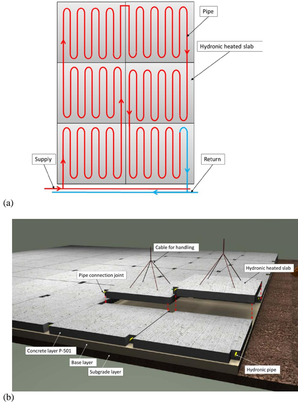
**Figure 5. Hydronic heated slabs assembly.**
