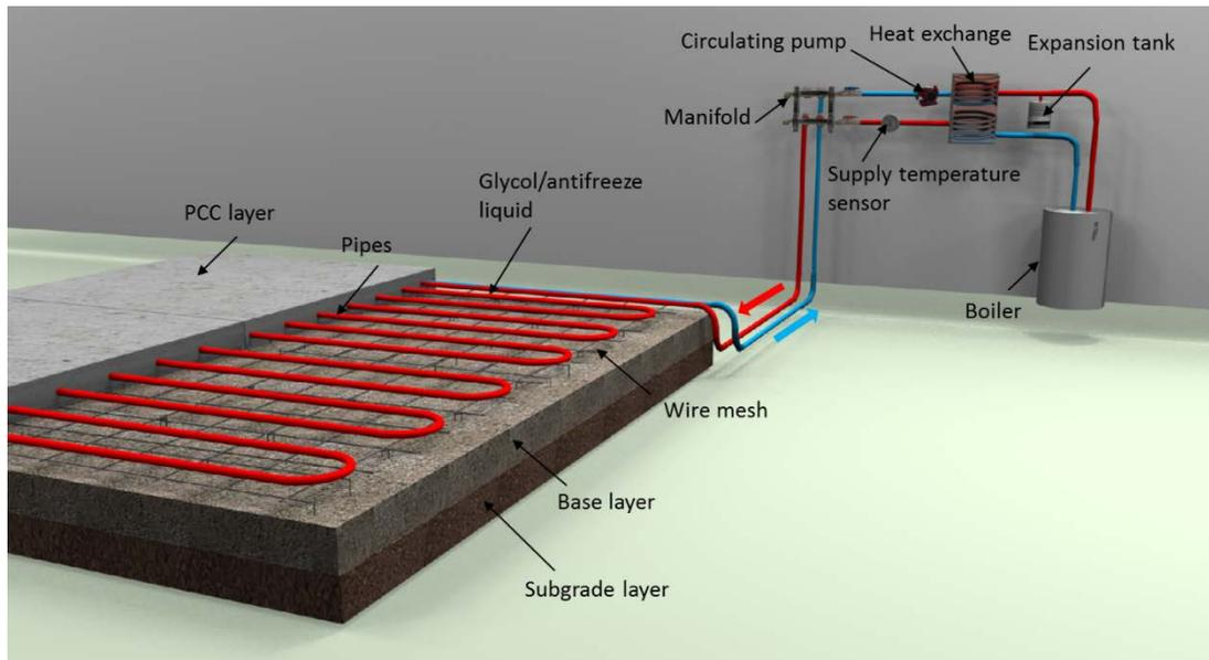
**Figure 1. Schematic of HHPS.**
