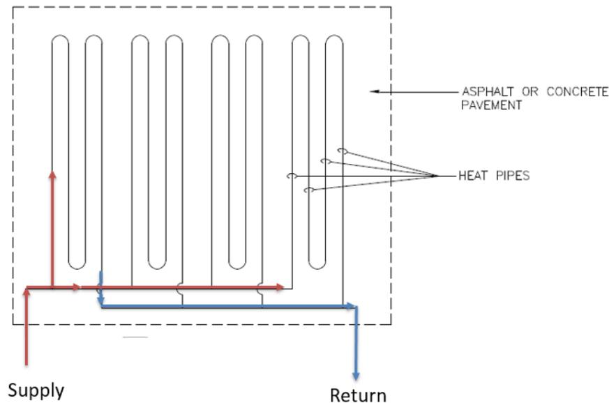
**Figure 2. Hydronic pipe pattern.**
