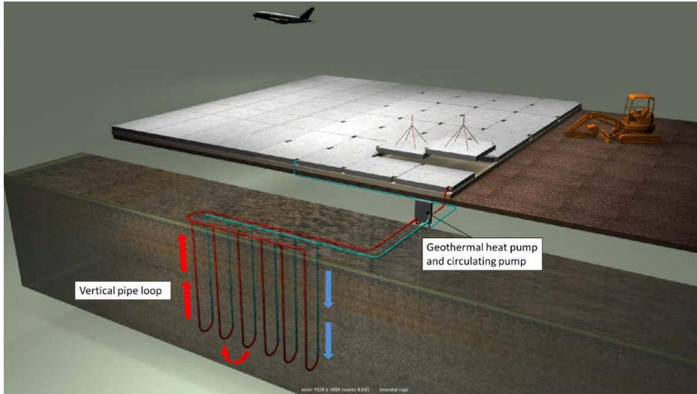
**Figure 6. HHPS with geothermal wells as heat source.**
