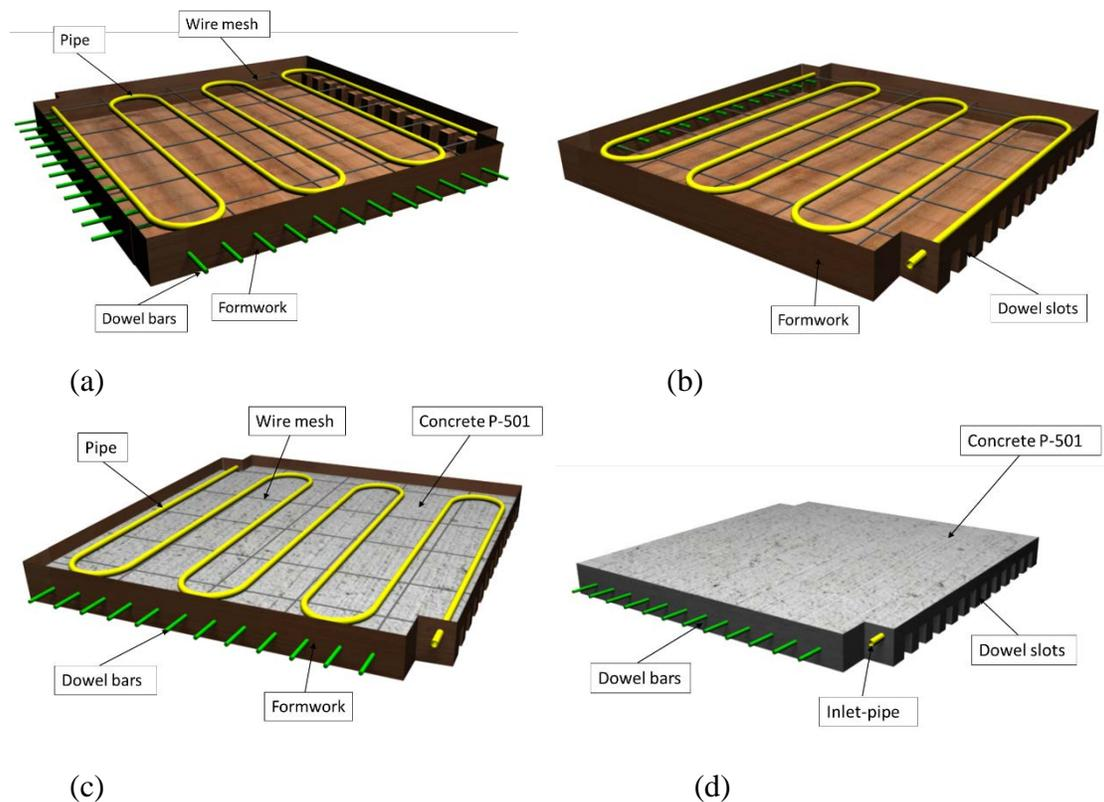
**Figure 4. Hydronic heated slab fabrication using PCP.**
