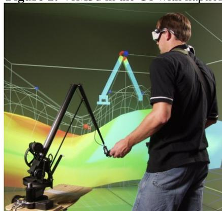
**3.1 Iterative re-analysis approach:** First, a model and its boundary conditions is loaded into the virtual world and a full stress analysis is performed. The resulting stress contours are displayed as a color contoured map in the part. As the model shape is altered, a two-stage approximation and reanalysis is performed to re-analyze for an updated stress state so changes may be evaluated quickly.
