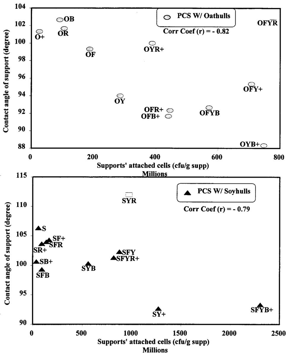
FIG. 2. Relationship between contact angle and *L. casei* biofilm population on various support (supp) surfaces during batch fermentation. The least significant difference ( $P < 0.05$ ) of contact angle and bacterial attachment were  $4.3^\circ$  and  $0.58 \times 10^9$  CFU/g of support, respectively. The empty squares were not included in the calculation of  $r$ . See Table 1 for support compositions.
