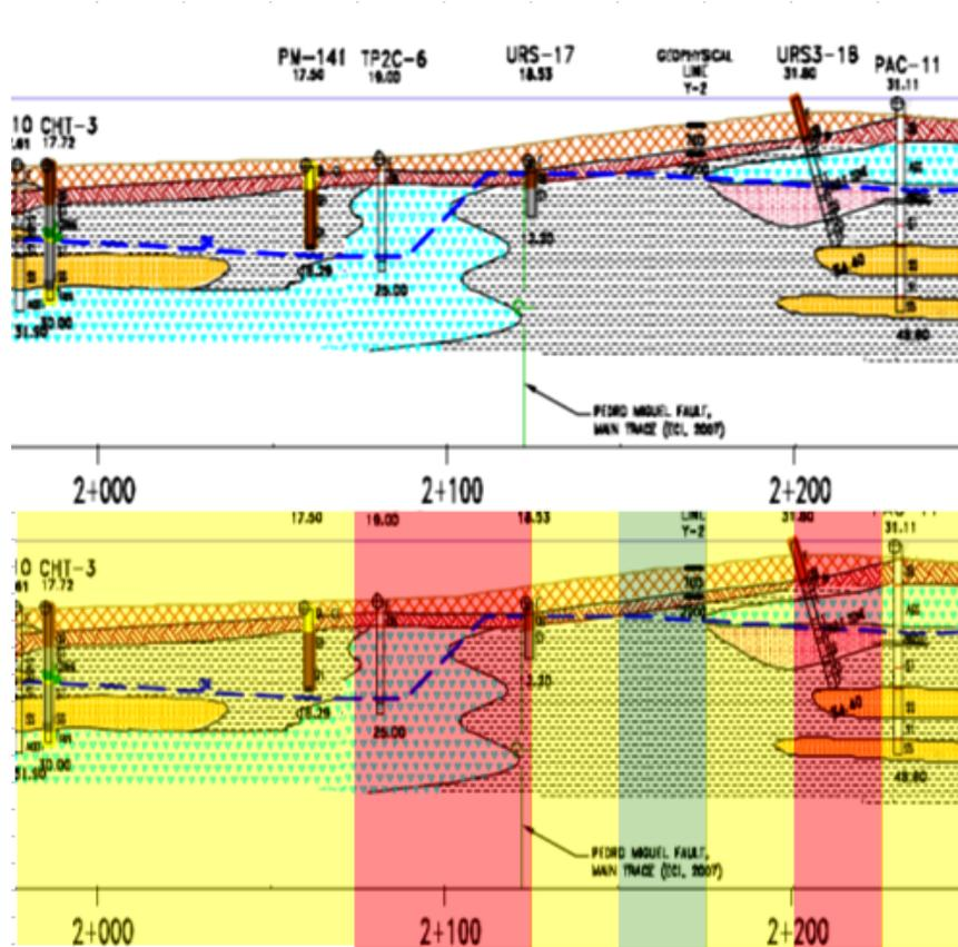
Figure 3 – Color coding for a section of the Borinquen Dam 1E foundation geological profile.
