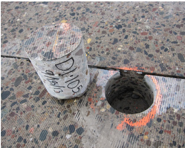
Sample core retrieved in 2013 showing the relationship to Joint 105 Cell 9
