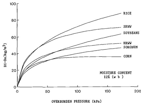
Figure 1—Variation in bulk density of six whole grains for a moisture content (wb) of 12% (Thompson et al., 1987).
