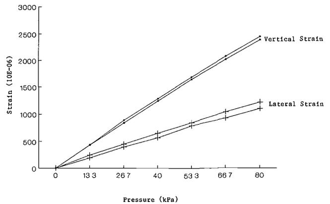
**Figure 2—Vertical and lateral strains of soft red winter wheat within a grain pressure apparatus using a diaphragm pressure cell.**
