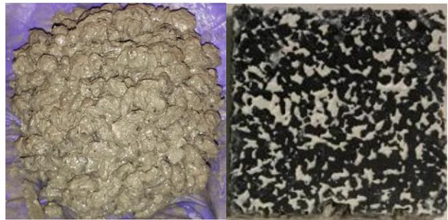
*Hand-formed ball of the pure Portland cement specimen for the workability test (left) and cross-section of the 15% fly ash specimen prepared for testing with the RapidAir method and the flatbed scanner method (right)*
