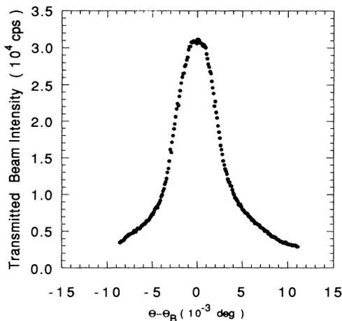
FIG. 3. Intensity of the forward diffracted beam ( $O$  beam) as the sample is rotated through the diffraction condition. The nominal zero of the horizontal scale was chosen at the center of the angular range of the reflection.
