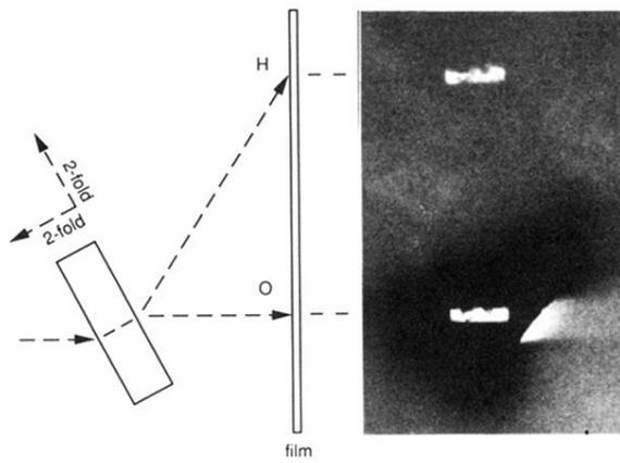
FIG. 2. A schematic of the configuration used to observe the Borrmann effect from Al-Pd-Mn. The photograph at right was taken 3.5 cm behind the sample and shows the *O*- and *H*-diffracted beams as well as the dark outline of the sample. The bright spot at the lower right resulted from spillover of the incident beam at the edge of the sample.
