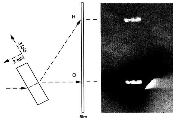
FIG. 2. A schematic of the configuration used to observe the Borrmann effect from Al-Pd-Mn. The photograph at right was taken 3.5 cm behind the sample and shows the  $O$ - and  $H$ -diffracted beams as well as the dark outline of the sample. The bright spot at the lower right resulted from spillover of the incident beam at the edge of the sample.
