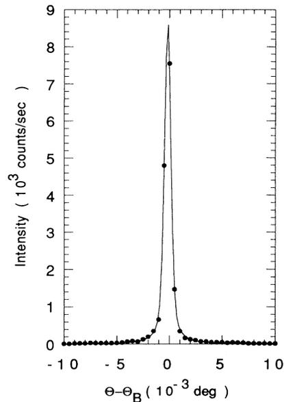
FIG. 1. Transverse scan ( $\theta$  scan) of the Al-Pd-Mn 8/12 peak. The solid line through the data is intended as a guide to the eye.
