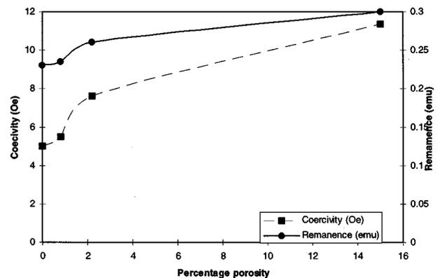
FIG. 3. Variation of coercivity and remanence with the density of nickel specimens with controlled amounts of porosity.
