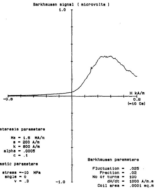
FIG. 4. Modelled Barkhausen signal amplitude under 10 MPa compression.
