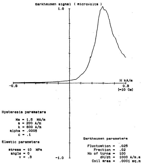
FIG. 3. Modelled Barkhausen signal amplitude under 10 MPa tension.
