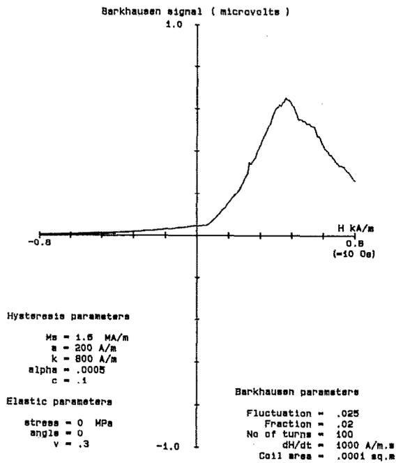
FIG. 2. Modelled Barkhausen signal amplitude under zero stress.
