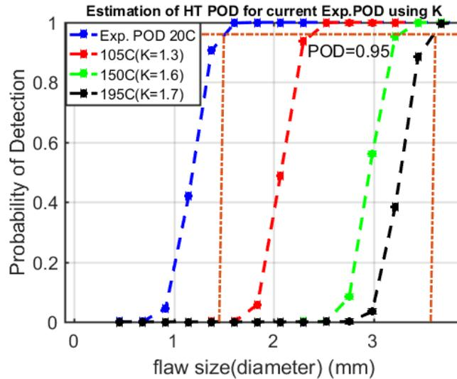
Fig. 10 Estimation of High temperature(HT) POD using room temperature experimental POD (dashed blue line) with temperature correction factor for PZT-5A, obtained from the physics based model
