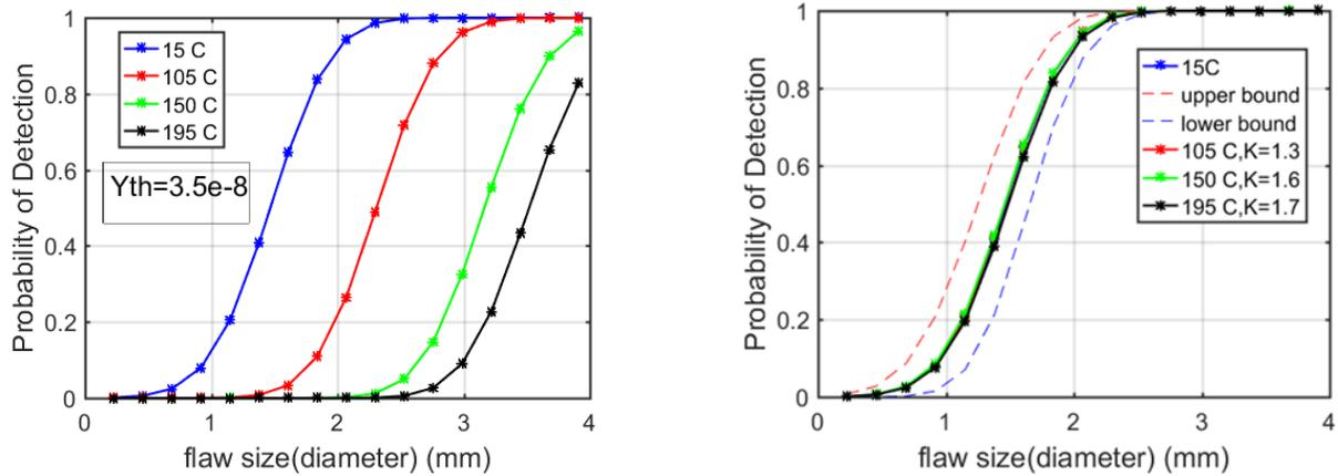
Fig. 9 Model based POD a) Without correction factor b) With PZT-5A temperature correction factor  $K$ . (dashed line (red, blue) indicate 95% confidence bounds for POD curve at 15 C
