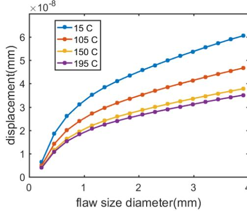
Fig. 5 Displacement versus flaw size (diameter) due to the temperature dependence of material coefficients of PZT-5A
