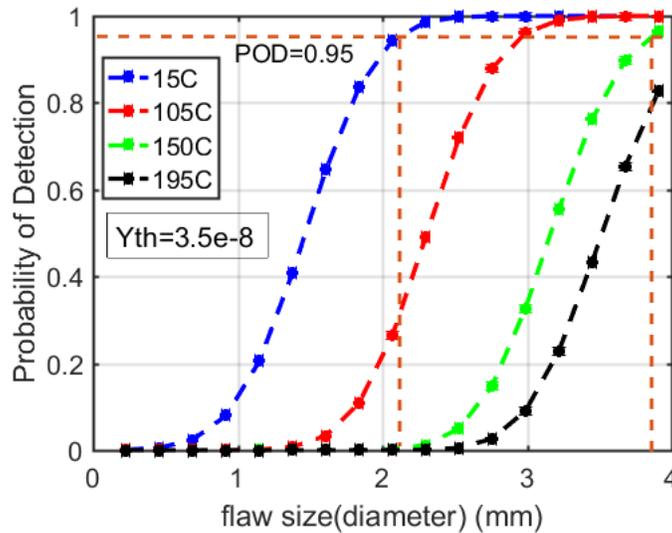
Fig. 8 Effect of temperature dependence of PZT -5A on the POD curve for a fixed threshold ( $Y_{th}$  at 15C) (orange dashed line showed flaw size at  $POD=0.95$  from 15C to 195C)
