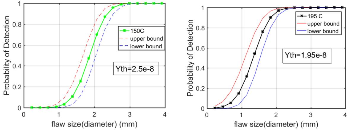
Fig. 7 Probability of detection at: (a) 150 C (b) 195 C for the predefined detection threshold  $Y_{th}$
