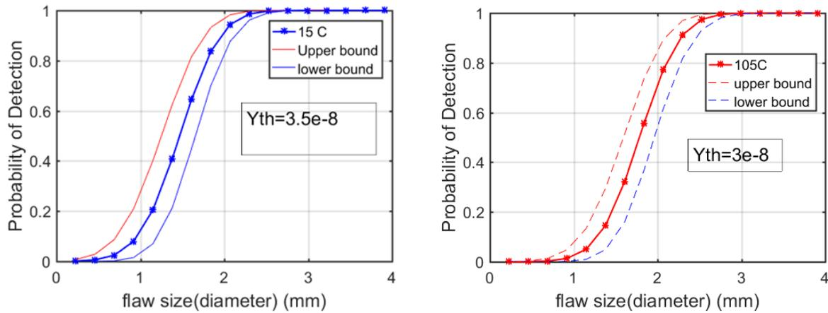
Fig. 6 Probability of detection: (a) 15 C (b) 105 C for the predefined detection threshold  $Y_{th}$
