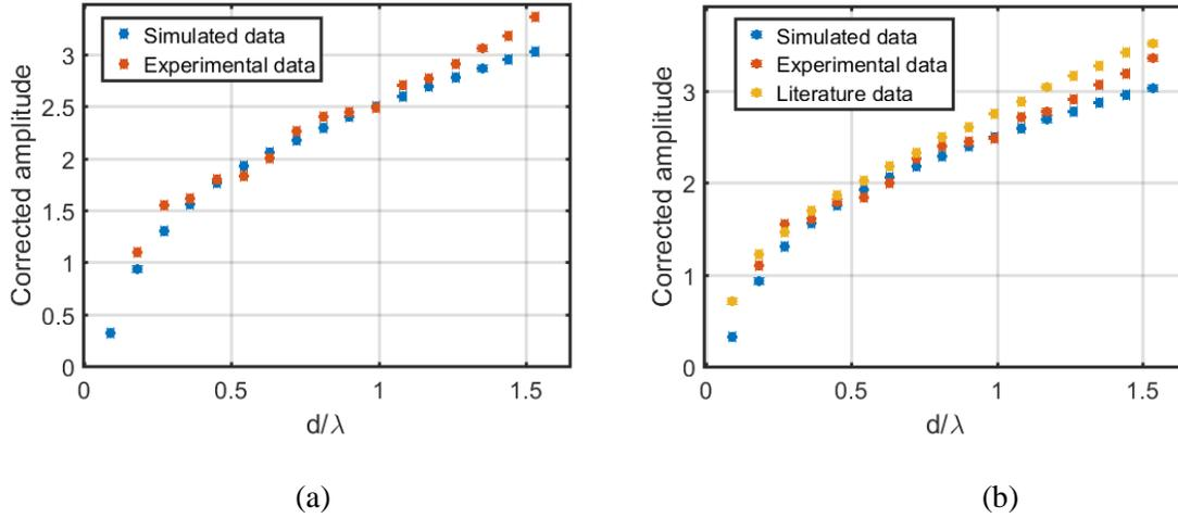
Fig. 4 (a-b) Comparison of corrected P-wave scattering amplitudes from simulation data, experimental data and previous published model data [31] for SDH
