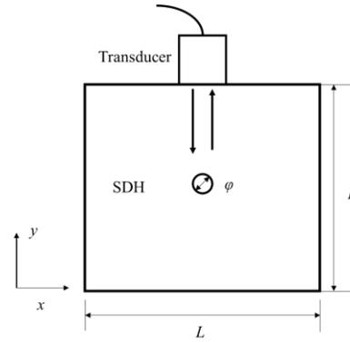
Fig. 2 Side drilled holes with diameter varying from 0.46mm to 3.9 mm in a 1018 low carbon steel block
