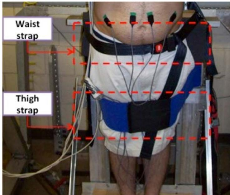
Figure 2. Lower extremity constraint in the lumbar dynamometer
