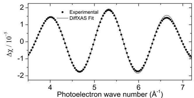
FIG. 3. Experimental DiffXAS Fe-K-edge spectra (solid) and its theoretical fit (dotted).
