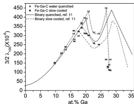
FIG. 1. MS of Fe–Ga–C alloys in the slow cooled and water quenched states compared with that of the binary Fe–Ga alloys. Trend lines are drawn to guide eyes.
