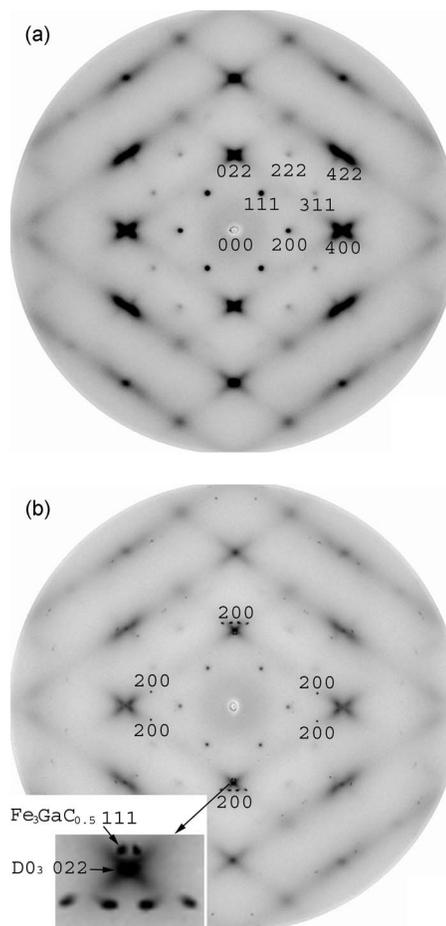
FIG. 3. Synchrotron x-ray results of Fe–26.7 at. % Ga–C alloy show the  $\text{D0}_3$  structure in both water quenched (a) and slow cooled (b) samples. The indexed spots in slow cooled sample (b) are from the (200) plane of the  $\text{Fe}_3\text{GaC}_{0.5}$  carbide; the enlarged portion shows the epitaxial relationship between the (022) plane of  $\text{D0}_3$  and (111) and (200) planes of  $\text{Fe}_3\text{GaC}_{0.5}$ .
