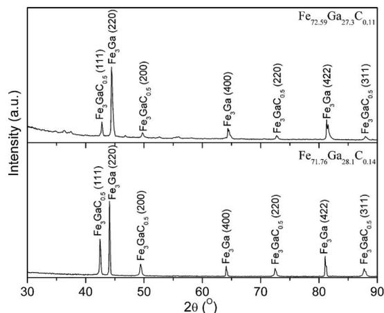
FIG. 2. XRD patterns show a mixture of  $\text{Fe}_3\text{GaC}_{0.5}$  and  $\text{Fe}_3\text{Ga}$  ( $\text{D0}_3$ ) phases in the  $\text{Fe}_{72.59}\text{Ga}_{27.3}\text{C}_{0.11}$  and  $\text{Fe}_{71.76}\text{Ga}_{28.1}\text{C}_{0.14}$  alloys.
