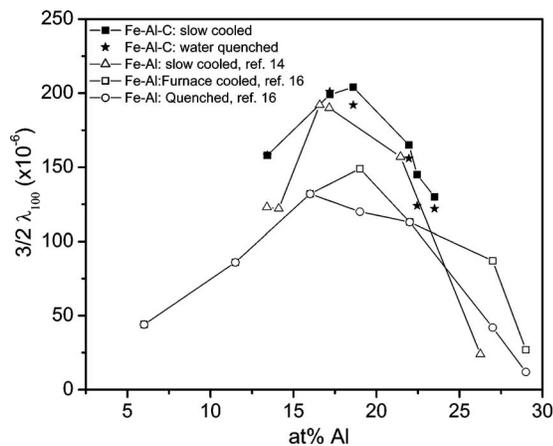
FIG. 4. MS of Fe–Al–C alloys compared with the binary Fe–Al alloys.
