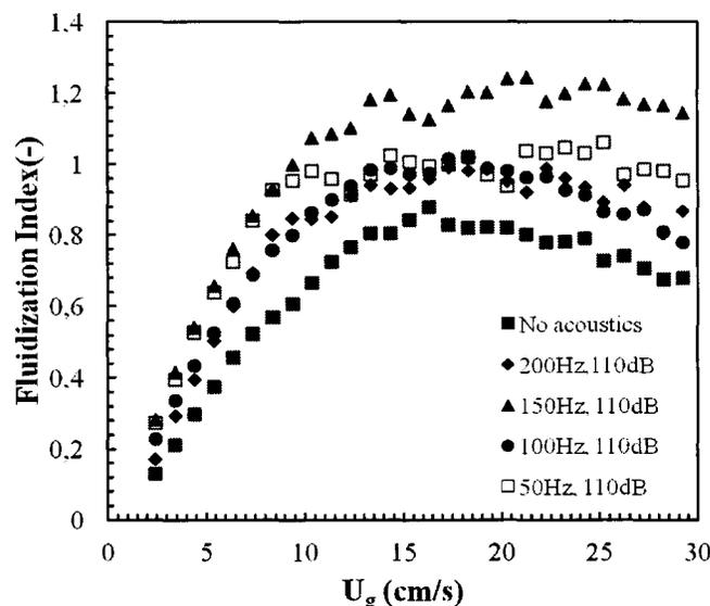
FIGURE 6: FLUIDIZATION INDEX AS A FUNCTION OF SUPERFICIAL GAS VELOCITY FOR GLASS BEADS 500-600  $\mu\text{m}$  AT  $H/D = 1$ .
