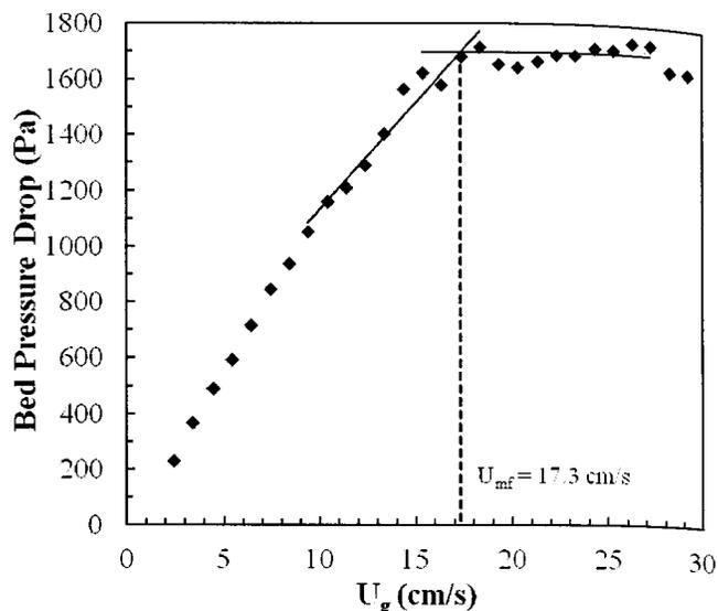
FIGURE 2: SAMPLE MINIMUM FLUIDIZATION PLOT FOR GLASS BEADS WITH  $H/D = 1$  (NO ACOUSTIC FIELD WAS APPLIED).
