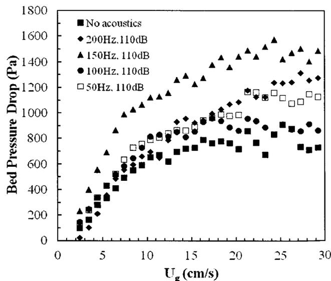
FIGURE 3: BED PRESSURE DROP AS A FUNCTION OF SUPERFICIAL GAS VELOCITY FOR 500-600  $\mu$ m GLASS BEADS AT  $H/D = 0.5$ .
