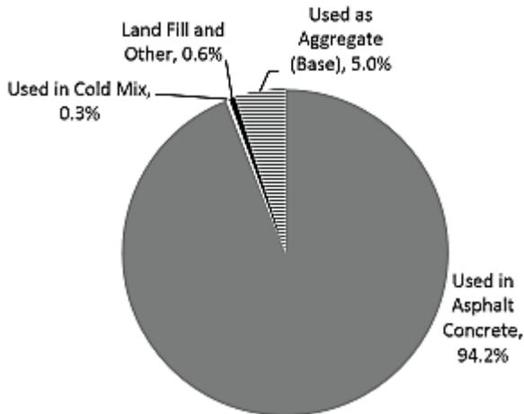
**Figure 1** Recycling and reuse statistics of asphalt materials [5].
