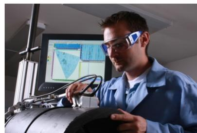
Fig 2. Phased array unit in use on a thick-wall polymer pipe, inspecting for lack of joint fusion [5].
