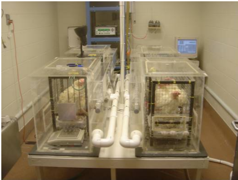
Figure 1a. An overview of the dynamic gas emissions chambers and measurement setup located in the Iowa State University Livestock Environment and Physiology (LEAP) Lab II.
