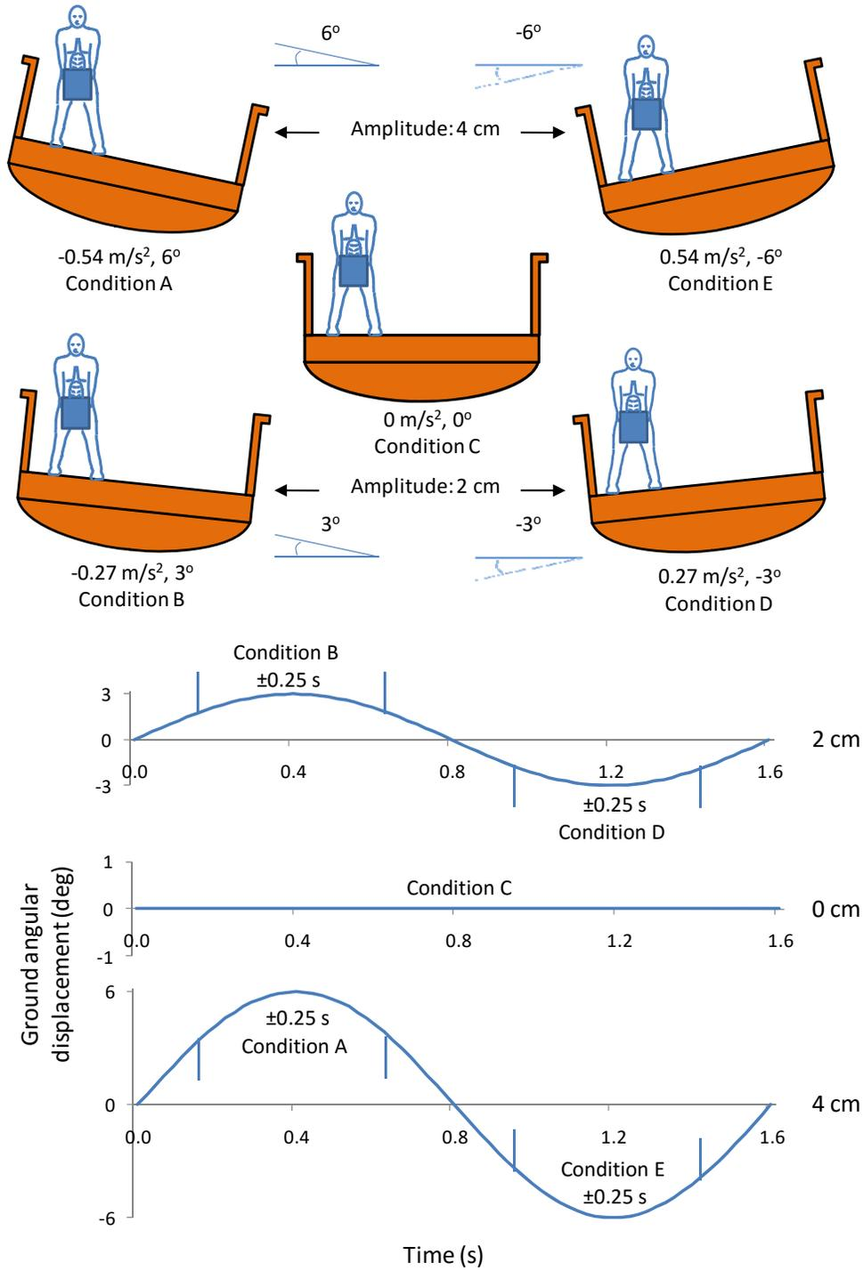
Figure 1: Coronal plane (front) view of the experimental set up and demonstration of the five ground surface conditions.
