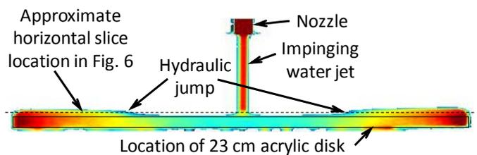
**FIGURE 5: VERTICAL SLICE OF THE 3D RECONSTRUCTED CT IMAGE THROUGH THE JET CENTERLINE FOR  $Re = 12000$ .**
