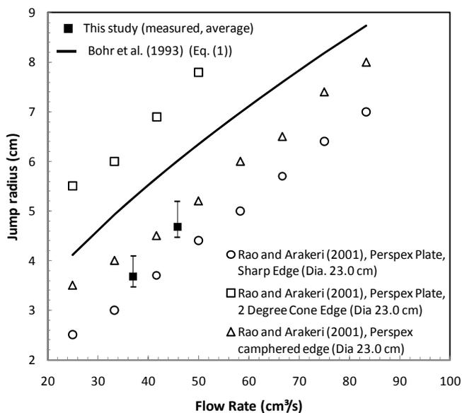
**FIGURE 8: HYDRAULIC JUMP RADIUS AS A FUNCTION OF JET EXIT FLOW RATE COMPARED TO BOHR ET AL. [8] (EQ. (1)) AND SELECTED DATA FROM RAO AND ARAKERI [3]. THE BARS ON THE MEASURED DATA POINTS REPRESENT THE RANGE FROM THE BEGINNING TO THE END OF THE HYDRAULIC JUMP, WHEREAS THE DATA POINTS ARE THE AVERAGE OF THE HALF-HEIGHT MEASUREMENTS**
