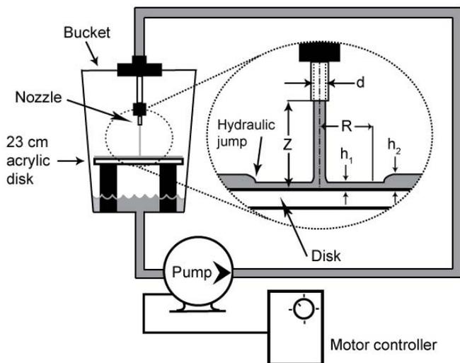
**FIGURE 1: SCHEMATIC LAYOUT OF THE EXPERIMENTAL SETUP WITH CLOSE-UP OF THE REGION OF INTEREST.**
