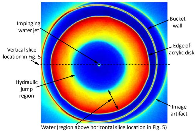
**FIGURE 6: HORIZONTAL SLICE OF THE 3D RECONSTRUCTED CT IMAGE THROUGH THE HYDRAULIC JUMP REGION FOR  $Re = 12000$ .**
