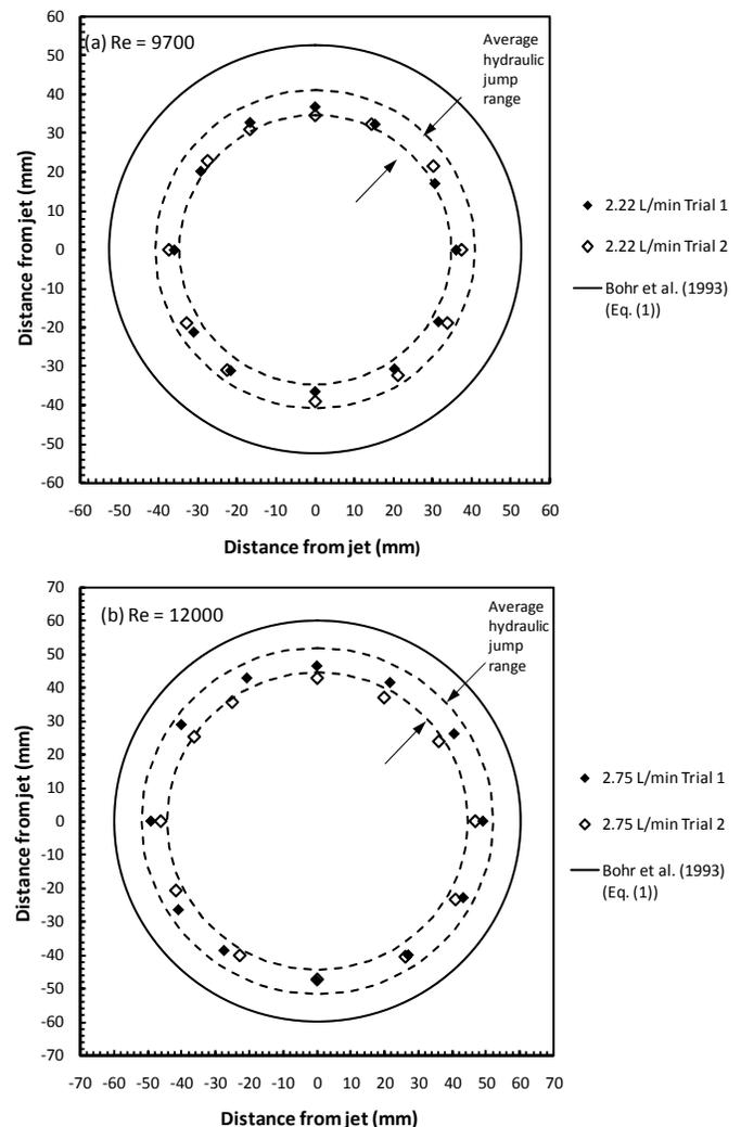
**FIGURE 7: HYDRAULIC JUMP RADII AS MEASURED FROM THE CT IMAGES ON THREE DIFFERENT HORIZONTAL PLANES FOR (a)  $Re = 9700$  AND (b)  $Re = 12000$ .**
