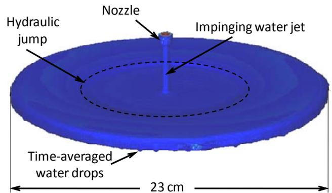
**FIGURE 4: RECONSTRUCTED 3D CT IMAGE OF THE IMPINGING WATER JET AND HYDRAULIC JUMP FOR  $Re = 12000$ .**
