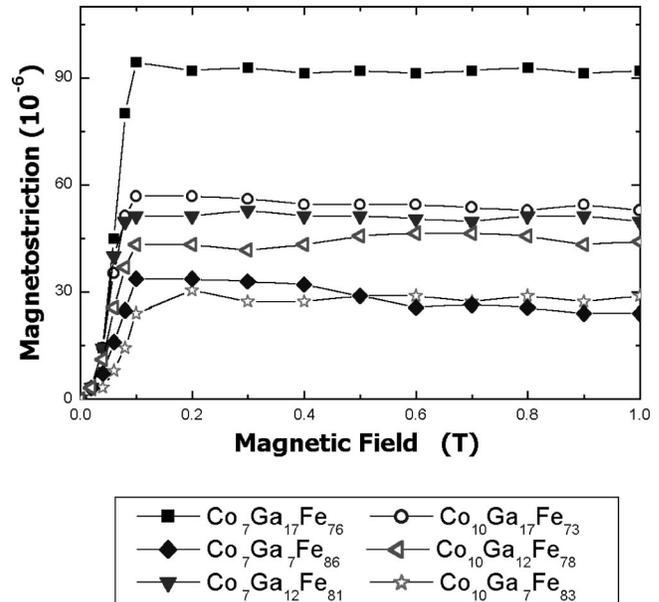
FIG. 4. Schematic of the magnetostriction changing with the magnetic field. The solid spots (square, triangle and circle) are the series of alloys with 7% cobalt; on the other hand, the open spots are the series of alloys with 10% cobalt. For larger percentages of cobalt, the magnetostriction actually decreases with Ga concentration.
