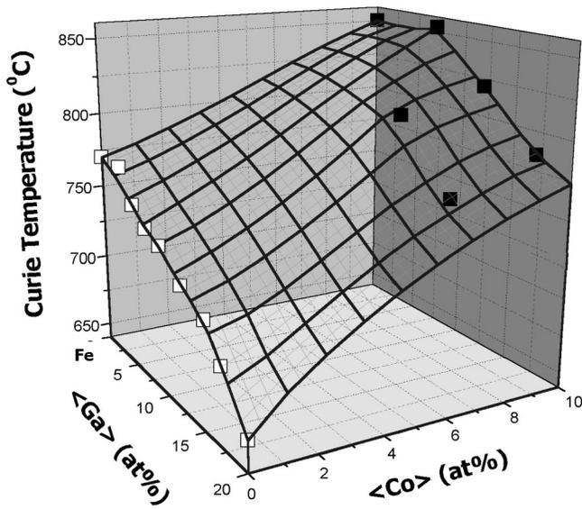
FIG. 1. Three-dimensional plot of the Curie temperature of the polycrystalline FeCoGa alloys. The solid squares are the experimental data. For comparing to the experimental data, the open squares are taken from the Fe–Ga phase diagram (see Ref. 6). The three-dimensional plot was fitted by both the experimental data and the calculated results.
