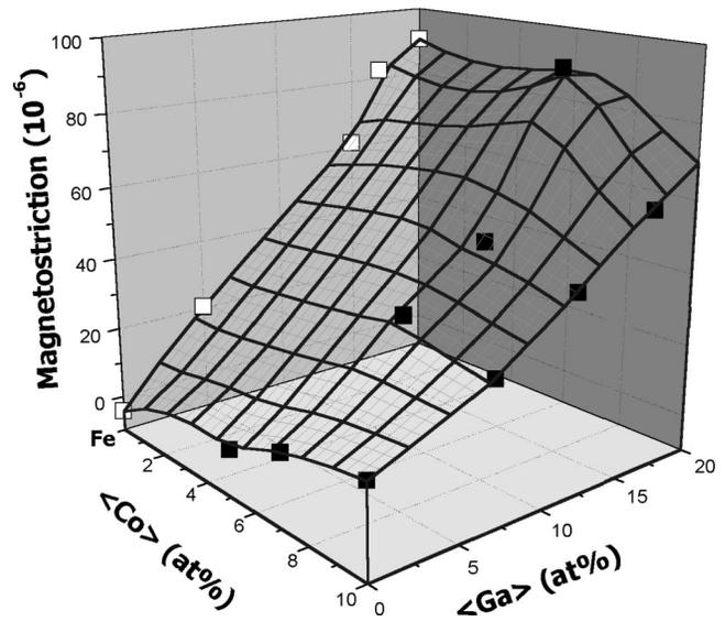
FIG. 3. Three-dimensional plot of the magnetostriction of the polycrystalline FeCoGa alloys. The solid squares are the experimental data. For comparing to the experimental data, the open squares are calculated results from the magnetostriction constants of FeGa single crystal,<sup>2</sup> i.e.,  $\lambda_s = 2\lambda_{100}/5 + 3\lambda_{111}/5$ .
