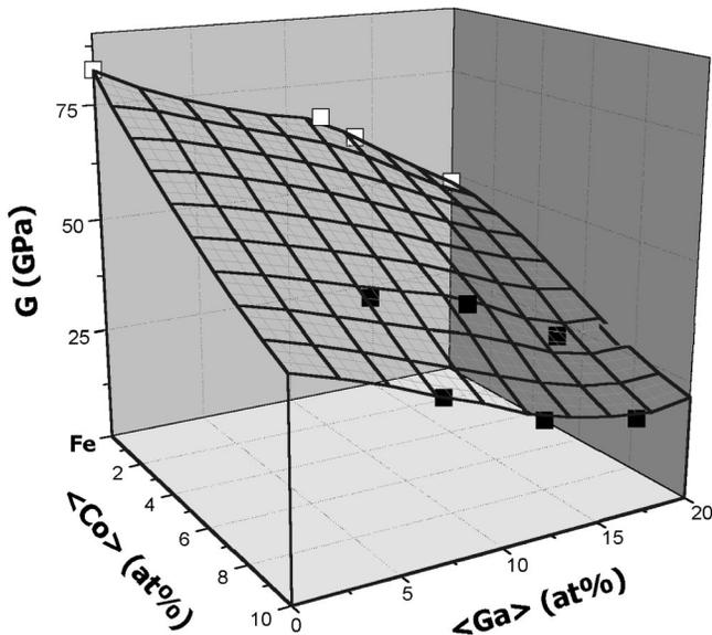
FIG. 2. The shear elastic moduli of the polycrystalline FeCoGa ternary alloys are schematically shown in a three-dimensional graph. The solid squares are the experimental data of these polycrystals. The opened squares are calculated results, which are data converted from the elastic constants of FeGa single crystals (see Ref. 7) by averaging the Reuss and Voigt approximations.
