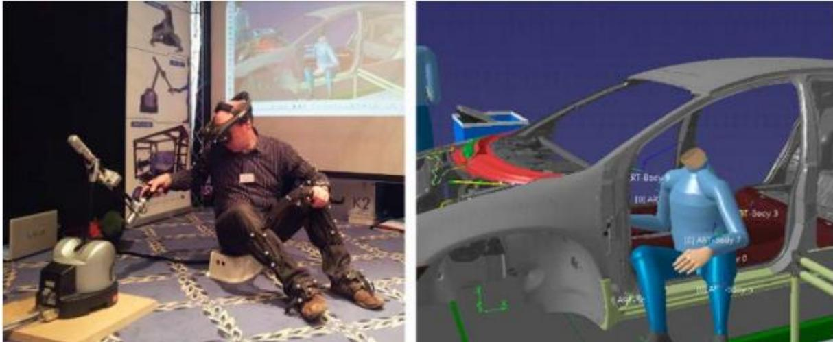
**Figure 6:** First author simulating an assembly operation inside a car. **Note:** The head of the human model is hidden in order to optimize the view through the head-mounted display.
