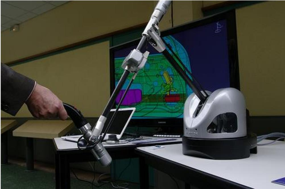
**Figure 4:** *Haptic device Virtuoso 6D*
