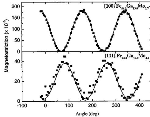
FIG. 2. Magnetostriction at 15 kOe of the  $\text{Fe}_{84.3}\text{Ga}_{13.0}\text{Mo}_{2.7}$  [(100) disk] sample and the  $\text{Fe}_{85.0}\text{Ga}_{10.2}\text{Mo}_{4.8}$  [(110) disk] sample. The solid lines represent fits to the data using the equation in the text.
