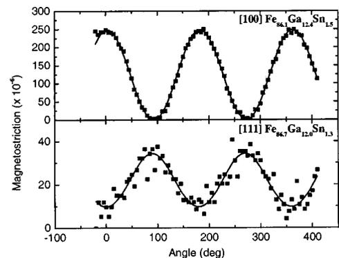
FIG. 3. Magnetostriction at 15 kOe of the  $\text{Fe}_{86.1}\text{Ga}_{12.4}\text{Sn}_{1.5}$  [(100) disk] sample and the  $\text{Fe}_{86.7}\text{Ga}_{12.0}\text{Sn}_{1.3}$  [(110) disk] sample. The solid lines represent fits to the data using the equation in the text.
