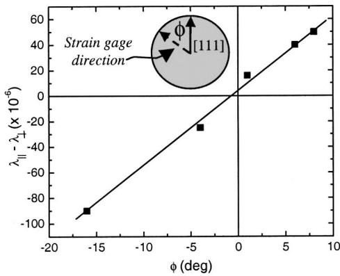
FIG. 1. Magnetostriction ( $\lambda_{||} - \lambda_{\perp}$ ) as a function of offset angle  $\phi$  of strain gage mounting relative to the  $[111]$  crystal axis for the  $\text{Fe}_{81.1}\text{Ga}_{16.2}\text{Ni}_{2.7}$  [(110) disk] sample.
